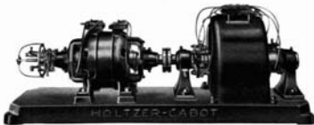
Fig. 13—Composite Multi-Cycle Motor Generator
