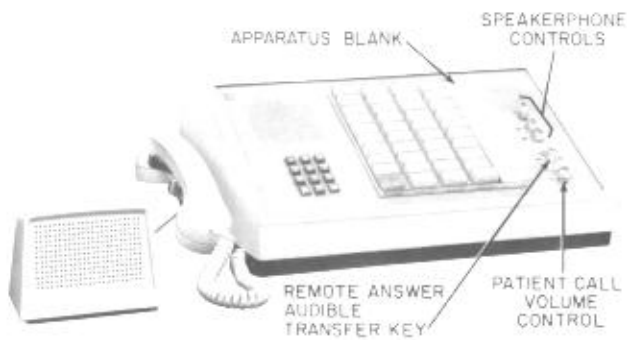
Fig. 3—J53038E, List 2 Console (TOUCH-TONE) With 760A Loudspeaker for Speakerphone
