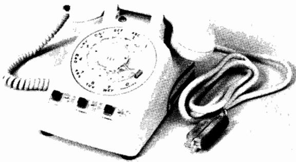
Figure 1. Type 576 Three-line desk telephone
