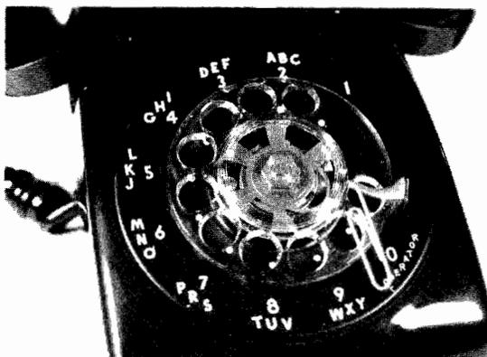
Fig. 3-2 REMOVING LUCITE FINGER PLATE
