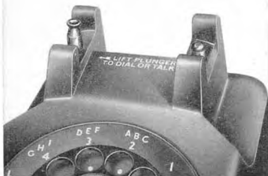
Fig. 3—500F Telephone Set Showing Plunger Switch and Instruction
