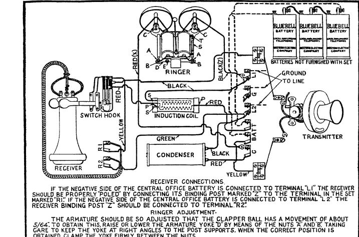
IF THE NEGATIVE SIDE OF THE CENTRAL OFFICE BATTERY IS CONNECTED TO TERMINAL "LI" THE RECEIVER SHOULD BE PROPERLY POLED" BY CONNECTING ITS BINDING POST MARKED "Z" TO THE TERMINAL IN THE SET MARKED "RI." IF THE NEGATIVE SIDE OF THE CENTRAL OFFICE BATTERY IS CONNECTED TO TERMINAL "L 2" THE RECEIVER BINDING POST "Z" SHOULD BE CONNECTED TO TERMINAL "R2."
