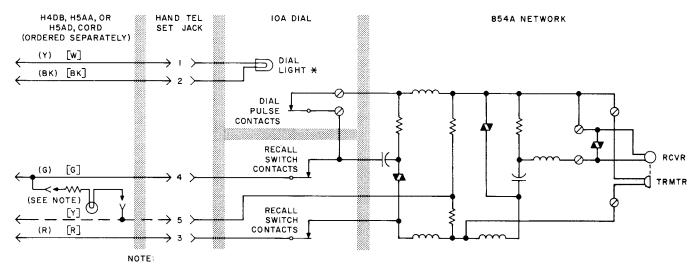
LAMP AND RESISTOR ARE PART OF H5AD CORD ONLY FOR MESSAGE WAITING FEATURE. [Y] LEAD IS NOT TERMINATED IN SET PLUG.
