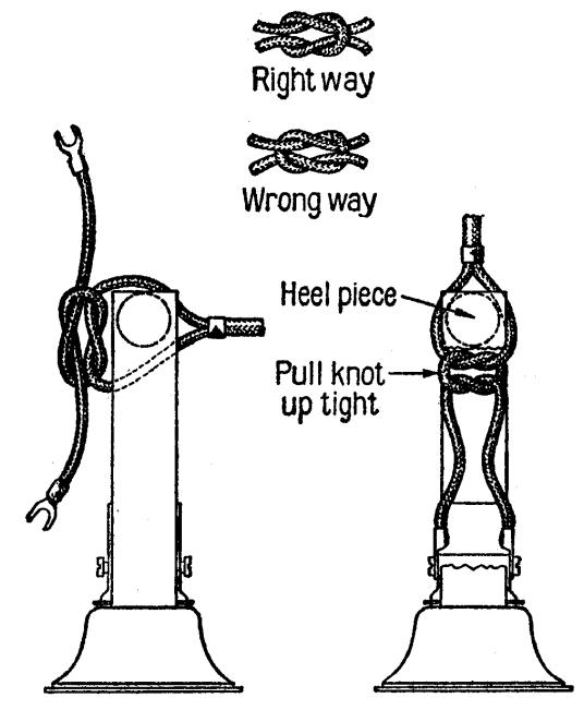
Pass one conductor on one side of heel piece and pass the other conductor on the other side of the heel piece. Tie with square knot, (see right way above), turn knot between limbs of magnet and insert spade tips under terminal screws.
