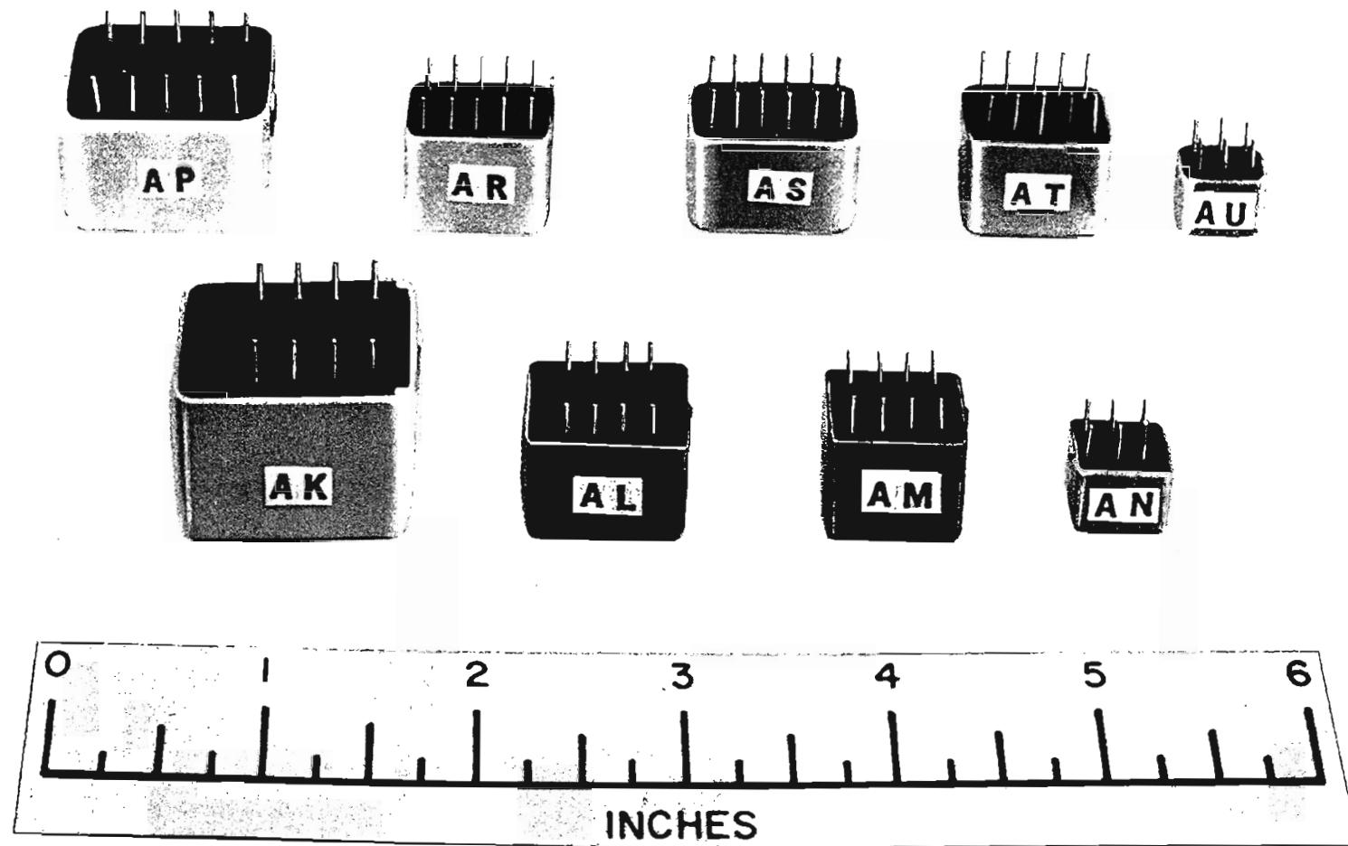
Fig. 5 Transmission Transformers AK to AU
