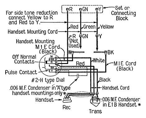
\*There must be a .006 MF condenser either in the handset or the handset mounting. There may be a condenser in both handset and mounting. Therefore, the E1B Handset (which has a condenser) may be used with any type of handset mounting but the E1A Handset (which has no condenser) must be used with the "A" type mountings only.
