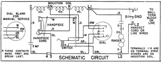
CONNECT GREEN RINGER LEAD TO TERMINAL L2 FOR BRIDGED RINGING; TO TERMINAL 5 FOR DIVIDED RINGING. USE 3-CONDUCTOR HANDSET CORD F-1205
