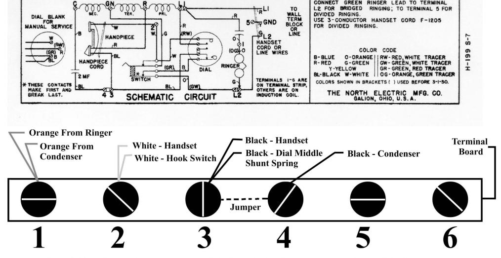
N.B. - A Soldered Jumper Between Terminals 3 & 4 is Normally Installed at the Factory on Bottom Side of Terminal Board
