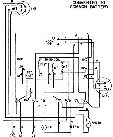
TO CONVERT TO COMMON BATTERY. DISCONNECT GEN. LEADS Y, W, B FROM 2,5,13 AND REMOVE GENERATOR. INSTALL DIAL BLANK OR DIAL. REMOVE GEN. COVER FROM TEL. CASE.
