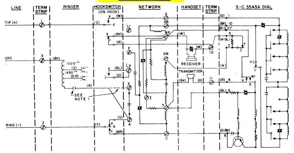
LINE POLARITY MUST BE OBSERVED
