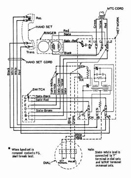
500C and D Telephone Sets-Connections
