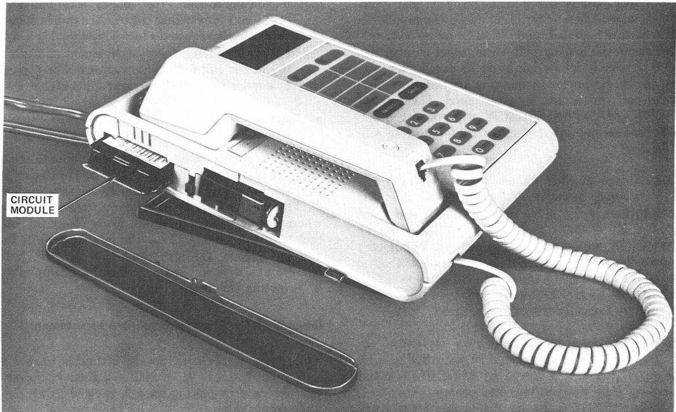
Fig. 2—Circuit Module Installation (Console)
