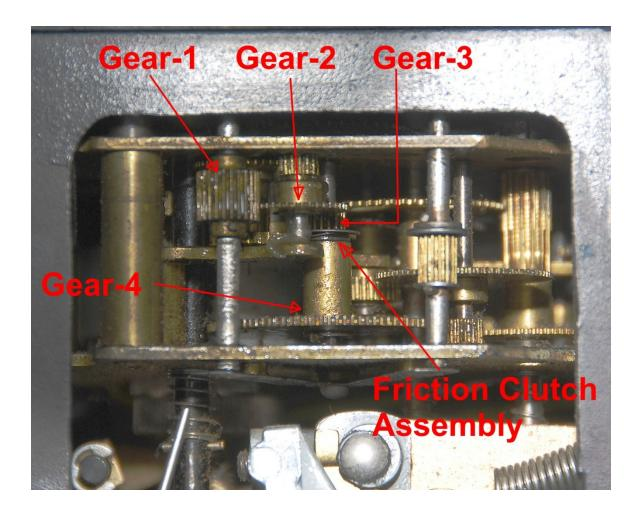
Insofar as the clock mechanism and workings are concerned, the various pivot points for all of the gears and shafts in the clock itself, can be lubricated with clock oil using a small pencil tipped artist's brush.
