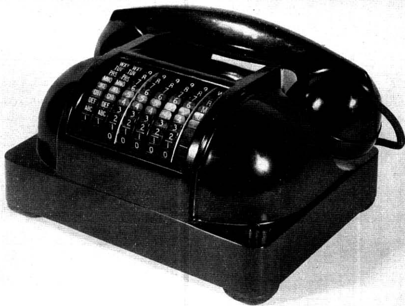
Fig. 5—Pre-set pulse-position-dialing telephone set.
