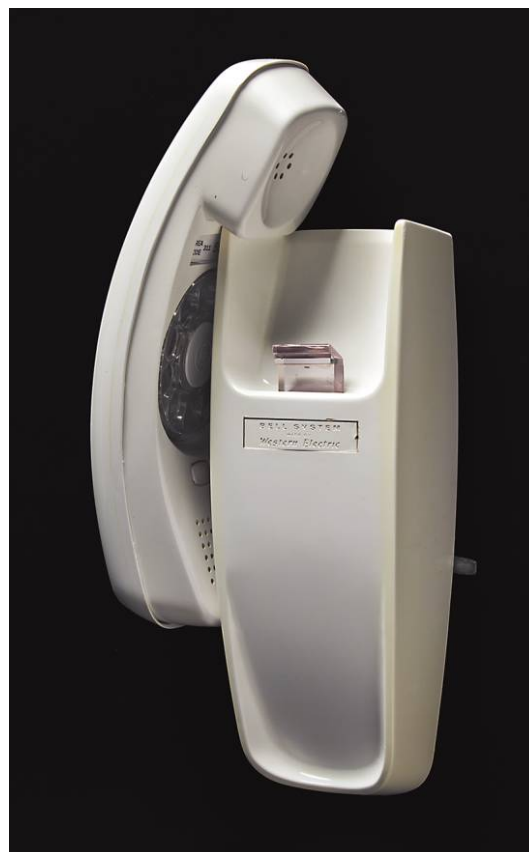
Fig. 47. Trimline off-hook handset on original wall-mounted base (AC1), 1965. (Gregg Museum of Art and Design.)
