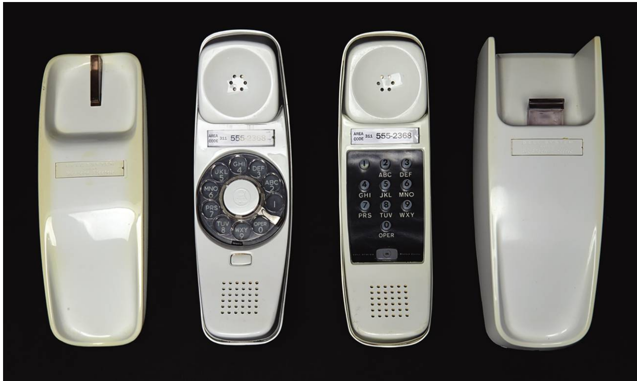
Fig. 44. Main components of early production Trimline telephones, showing (left to right) desk base, rotary handset, touchtone handset, and wall base, 1965–66. (Gregg Museum of Art and Design.)
