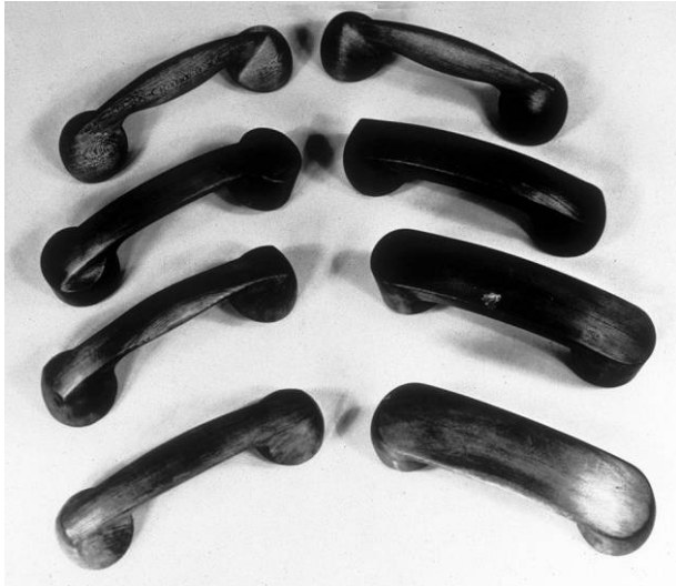
Fig. 21. Wooden handset prototypes showing F-type handset at upper left and Hose's original concept at right, third from top, ca. 1947. (Henry Dreyfuss Associates.)
