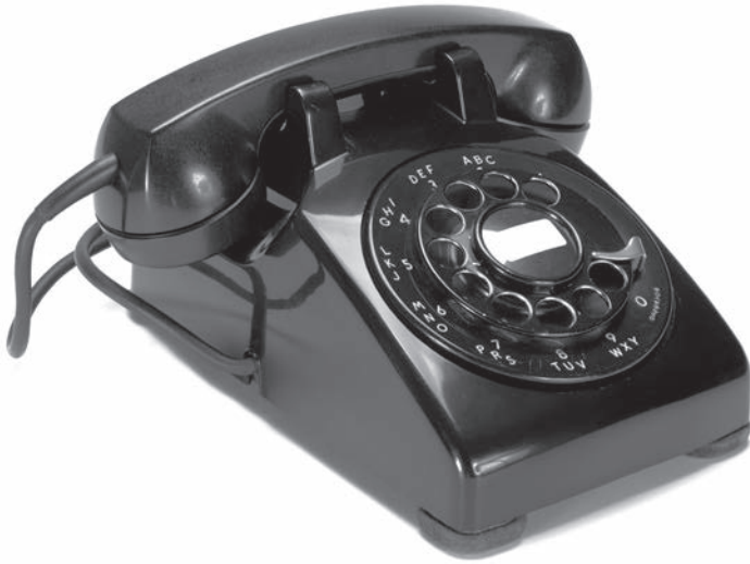
FIGURE 21.1 Western Electric No. 500 telephone introduced in 1949. (Photo by Matthew Gay, courtesy of the Gregg Museum of Art & Design, North Carolina State University.)
