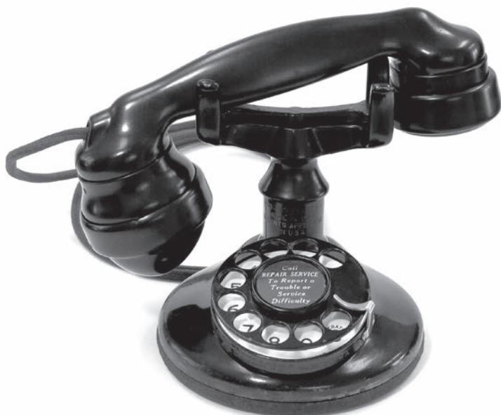
FIGURE 12.2 Western Electric Type E handset and A-type base of early 1927 with receiver-off-hook error.
