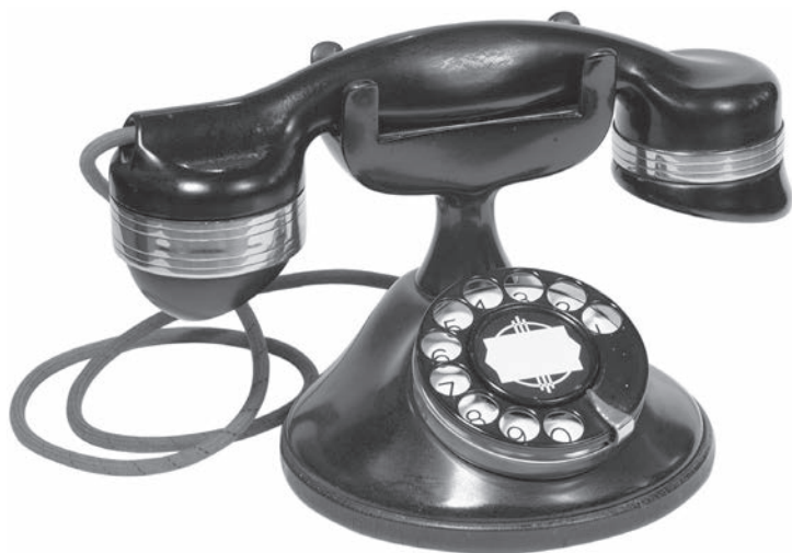
FIGURE 15.1 Automatic Electric No. 1 Monophone desk stand, 1925. (Photo by Marketa Ebert.)
