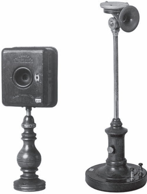
FIGURE 5.1 Blake transmitter, 1878 (left), and long-distance transmitter, 1885 (right), on desk stands (Photos courtesy of the AT&T Archives and History Center.)
