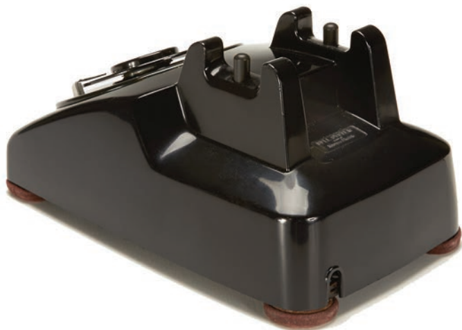
FIGURE 21.4 Rear view of the Western Electric No. 500 telephone showing the handhold cavity beneath the cradle. (Photo by Matthew Gay, courtesy of the Gregg Museum of Art & Design, North Carolina State University.)
