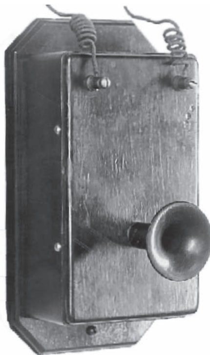
FIGURE 2.8 Bell's 1877 wall-mounted box telephone used as a transmitter. (Photo courtesy of the AT&T Archives and History Center.)
