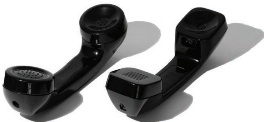
FIGURE 26.2 Comparison of the Type G (left) and Type K (right) handsets. (Photo by Ted Mueller.)
