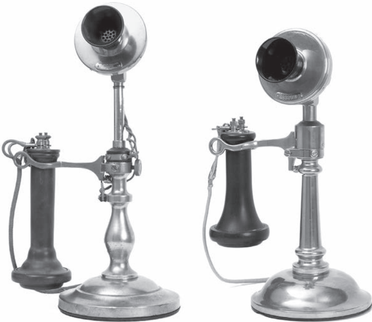
FIGURE 5.2 White's solid-back transmitter on desk stands, 1895 (left) and 1902 (right). (Photos by Matthew Gay.) TCI Library: www.telephonecollectors.info
