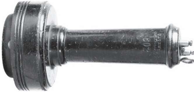
FIGURE 2.3 Bell Company hand telephone, June 1877. (Photo courtesy of the Division of Work and Industry, National Museum of American History, Smithsonian Institution.)
