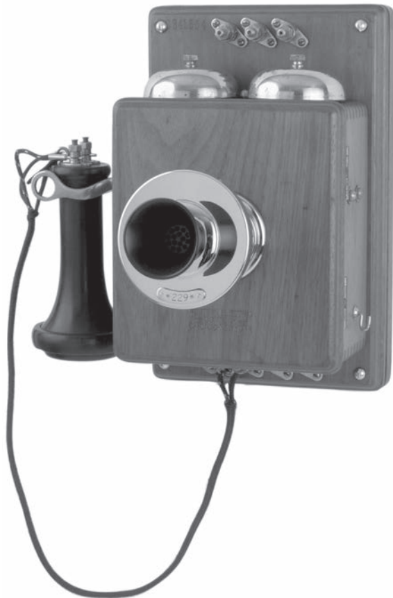
FIGURE 6.2 Western Electric's first wall phone with the booster circuit, ca. 1900. (Photo by Marketa Ebert.)
