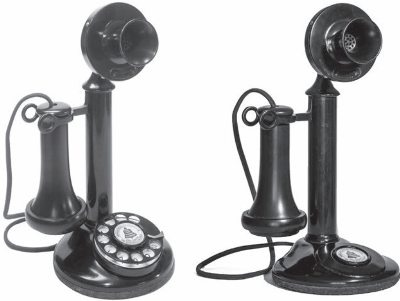
FIGURE 7.5 Desk stand with off-center shaft to accommodate a dial, ca. 1920. (Photos by Carroll Haugh and Ted Mueller.)
