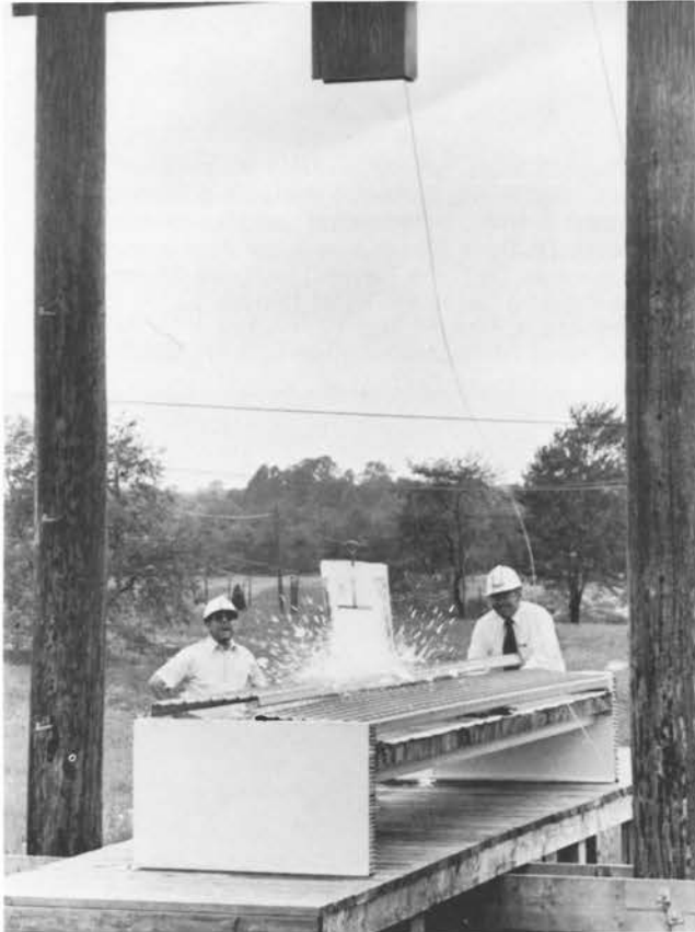
Falling ice. A block of ice falls 50 feet onto a prototype roof shield, as Vinnie Di Lullo (left) and Don Graupner conduct a test to evaluate the shield's effectiveness in protecting repeater huts from ice falling from microwave antenna structures.
