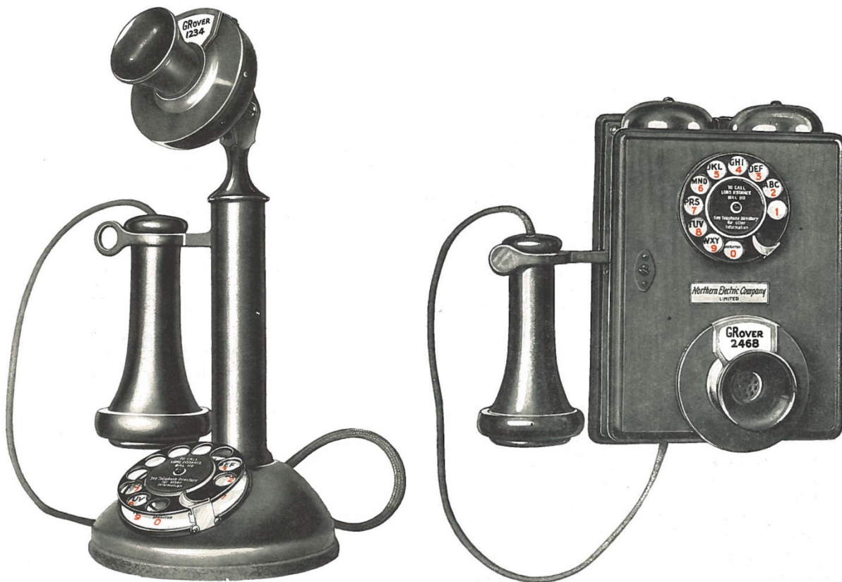
Dial desk stand and dial wall telephone used by Grover subscribers after cutover
