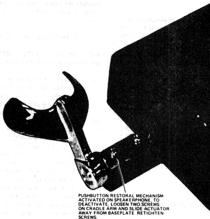
Figure 5. Pushbutton Restoral Mechanism (Wall Version).
