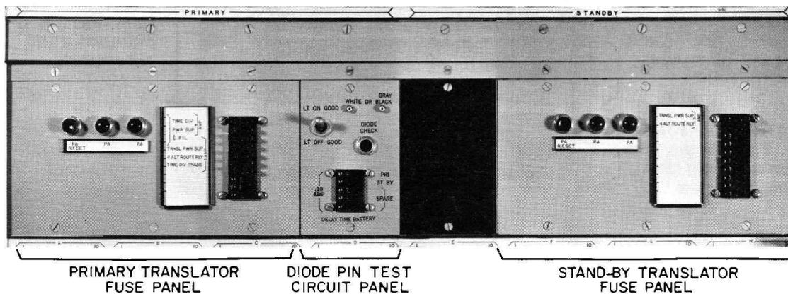
Figure 13. Fuse and Control Panel ("B" and "C" Translators).
