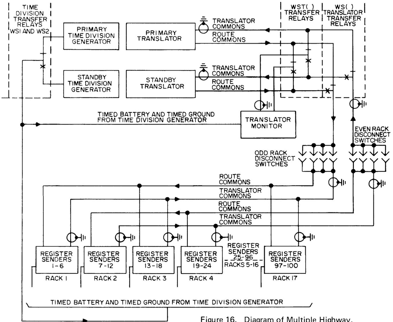
Figure 16. Diagram of Multiple Highway.
