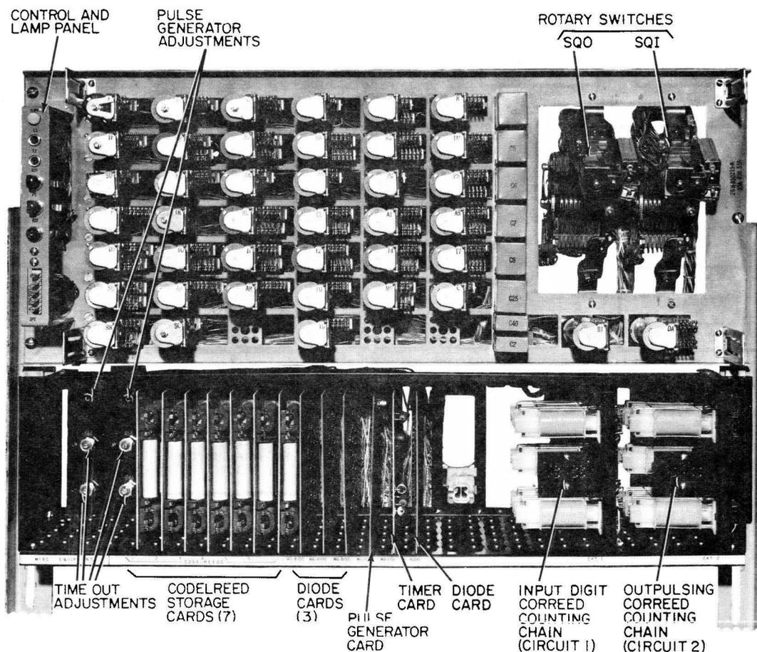
Figure 5. Register-Sender (H-850215-A).
