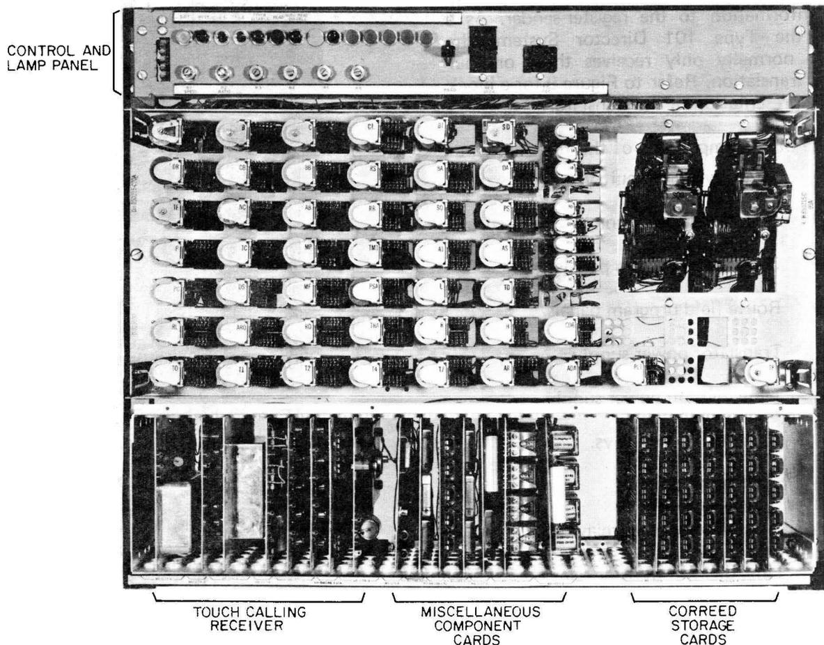
Figure 7. Register-Sender (H-850215-C).
