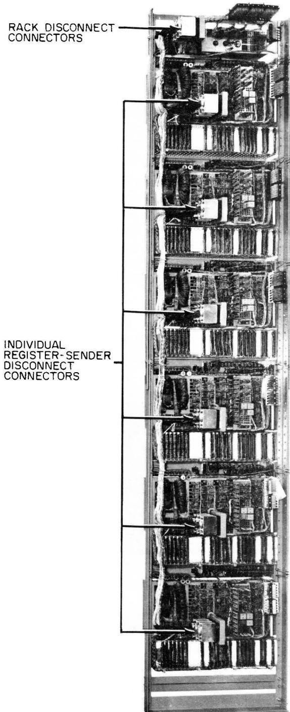
Figure 17. Type "C" Register-Sender Rack (Rear View).
