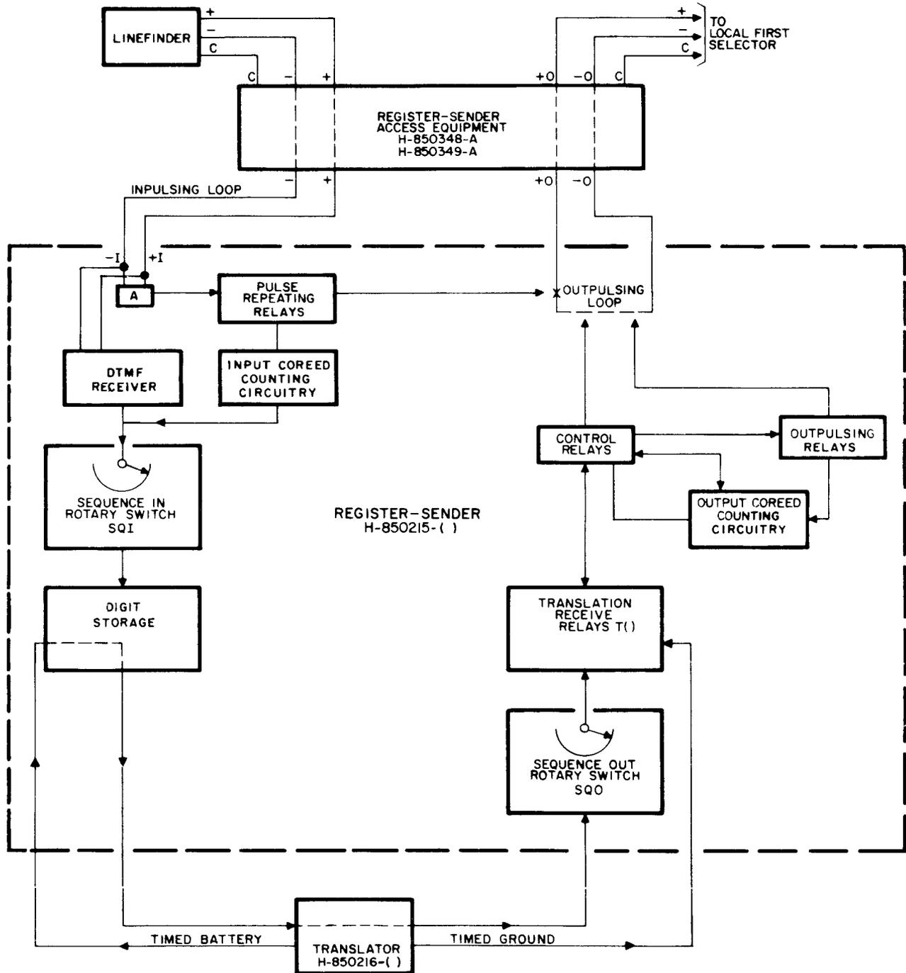
Figure 4. Register-Sender Block Diagram.
