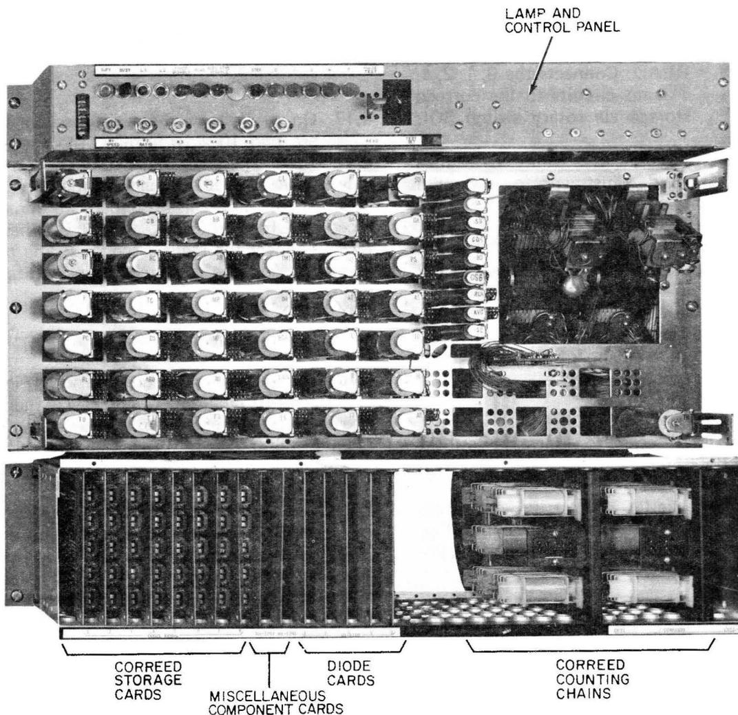
Figure 6. Register-Sender (H-850215-B).
