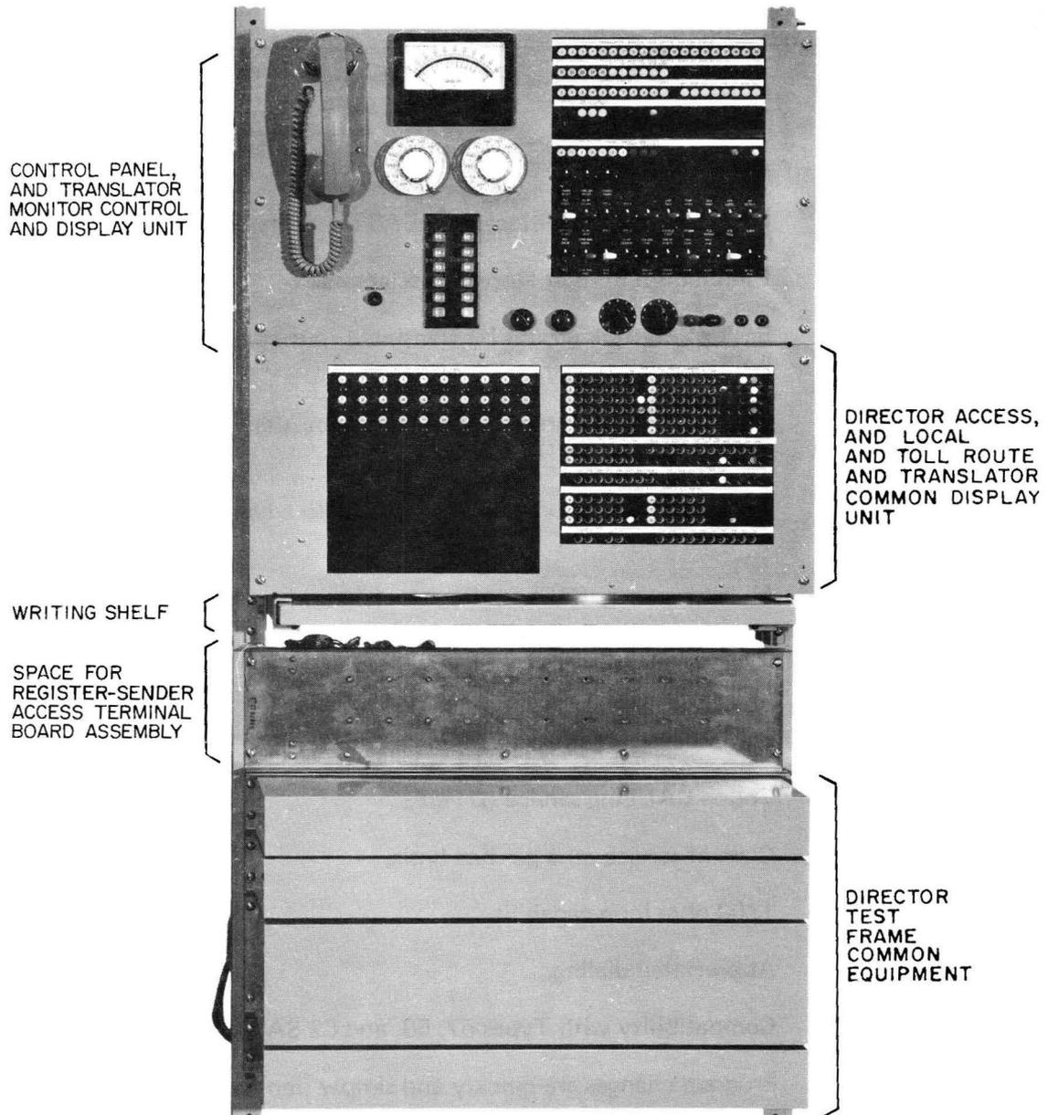
Figure 20. Typical Test Frame Used With Series 100 Director Systems.
