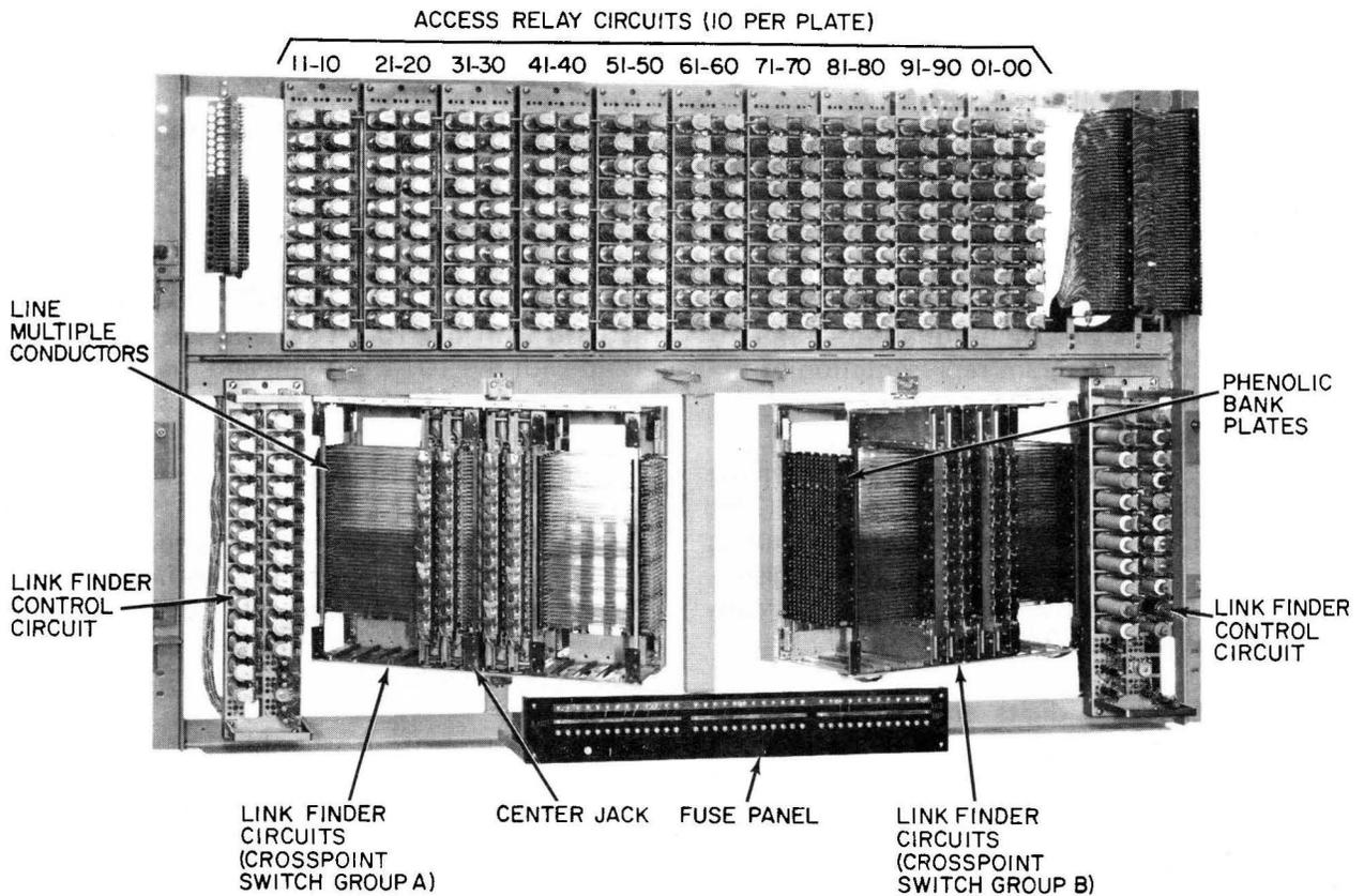
Figure 2. Register-Sender Access Equipment Shelf.
