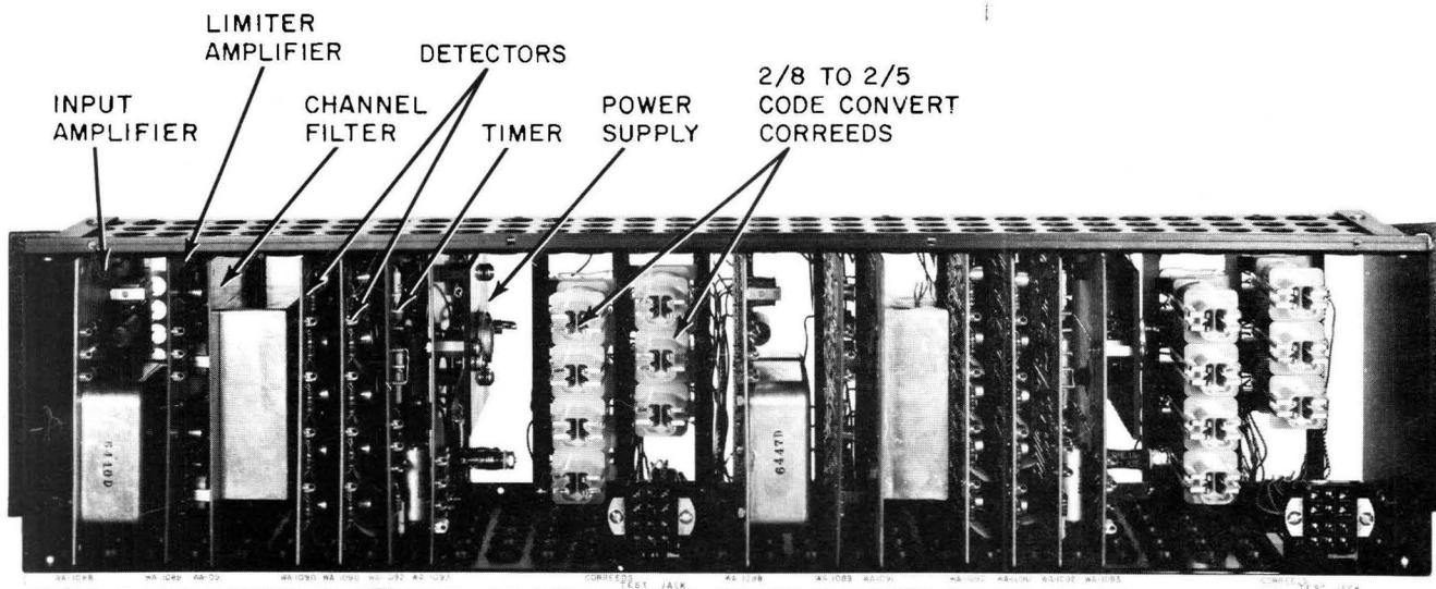
Figure 18. Card File, Two Touch Calling Receivers Mounted.
