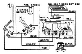
NOTE: WHEN 1182-A TEL. IS USED WITH 1156 BELL BOX CONNECT RED OF LINE CORD TO L-2 AND YEL-LOW OF LINE CORD TO 2-R.
