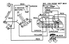
NOTE: FOR SIDE TONE REDUCTION REVERSE RED AND YELLOW CONDUCTORS ON CONNECTING RACK
