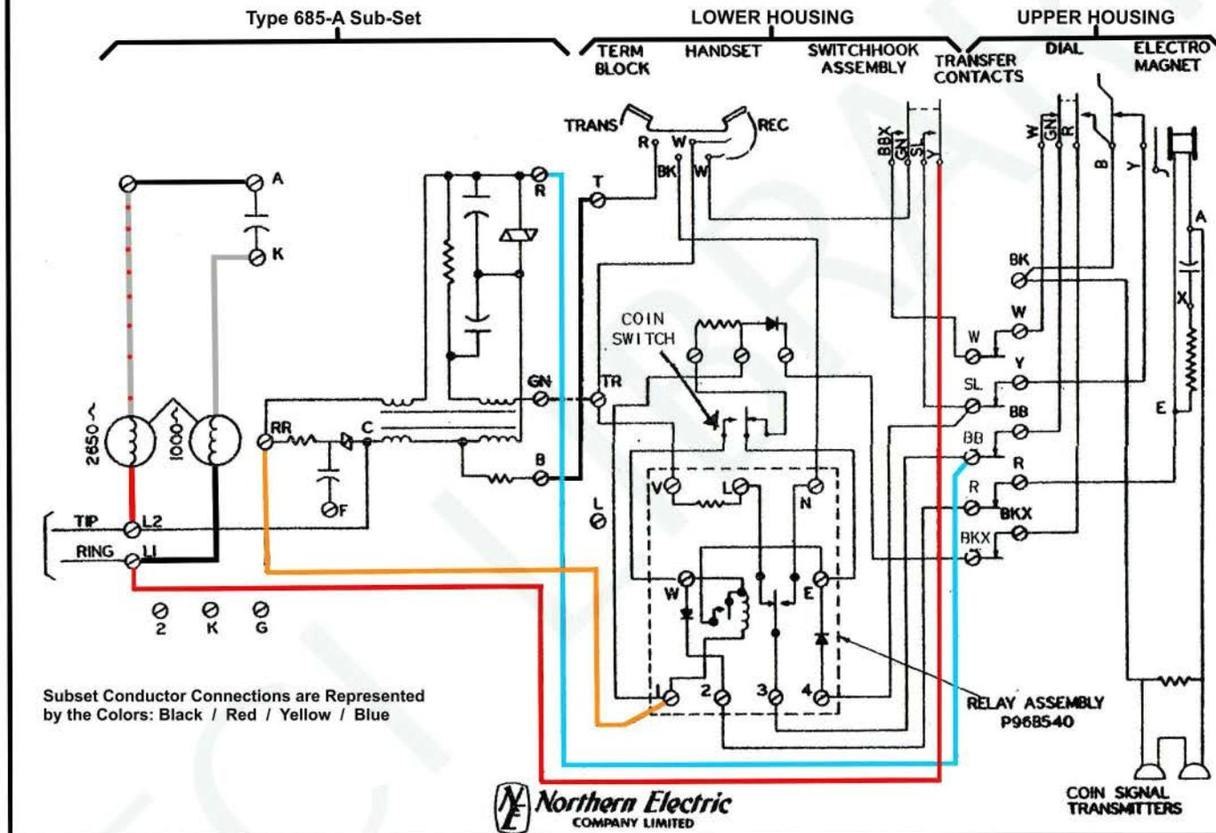
Fig. 3 - Circuit Diagram for Connecting QSD3A Coin Collector to NE-685A Network Type Subset
