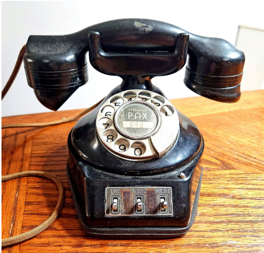
Automatic Electric AA-22 3-key, 2-line Monophone Cradle Telephone (Rick Saint photo)
