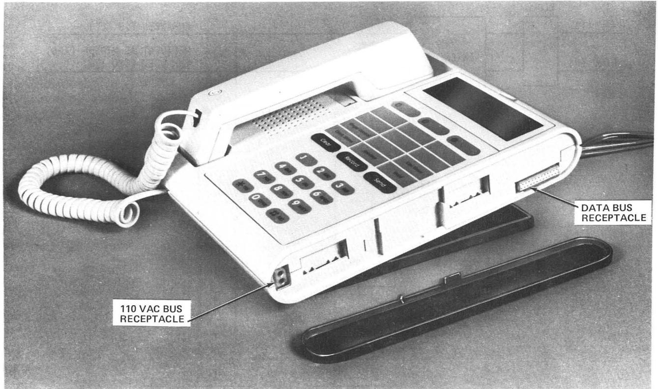
Fig. 6—Console With Right Cap Removed
