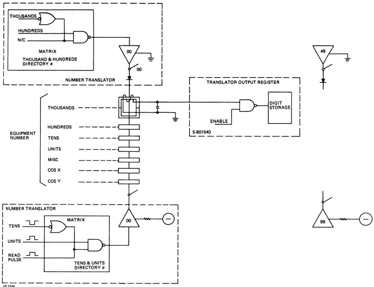
Figure 17. Example of a Directory Number to Equipment Number Translator
