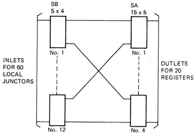
NOTE: 70 JUNCTORS CAN BE ACCOMMODATED BY ADDING 3 SB-STAGE SWITCHES
