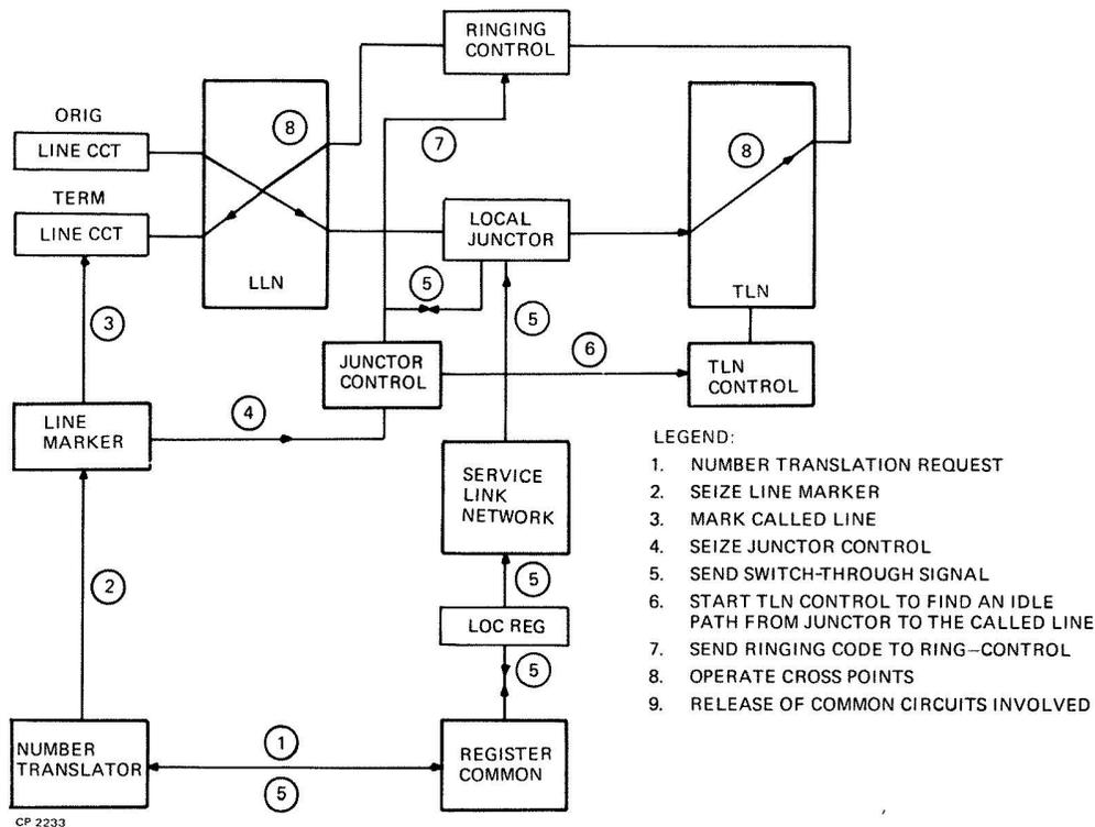
Figure 26. Termination of a Local Call, Functional Diagram
