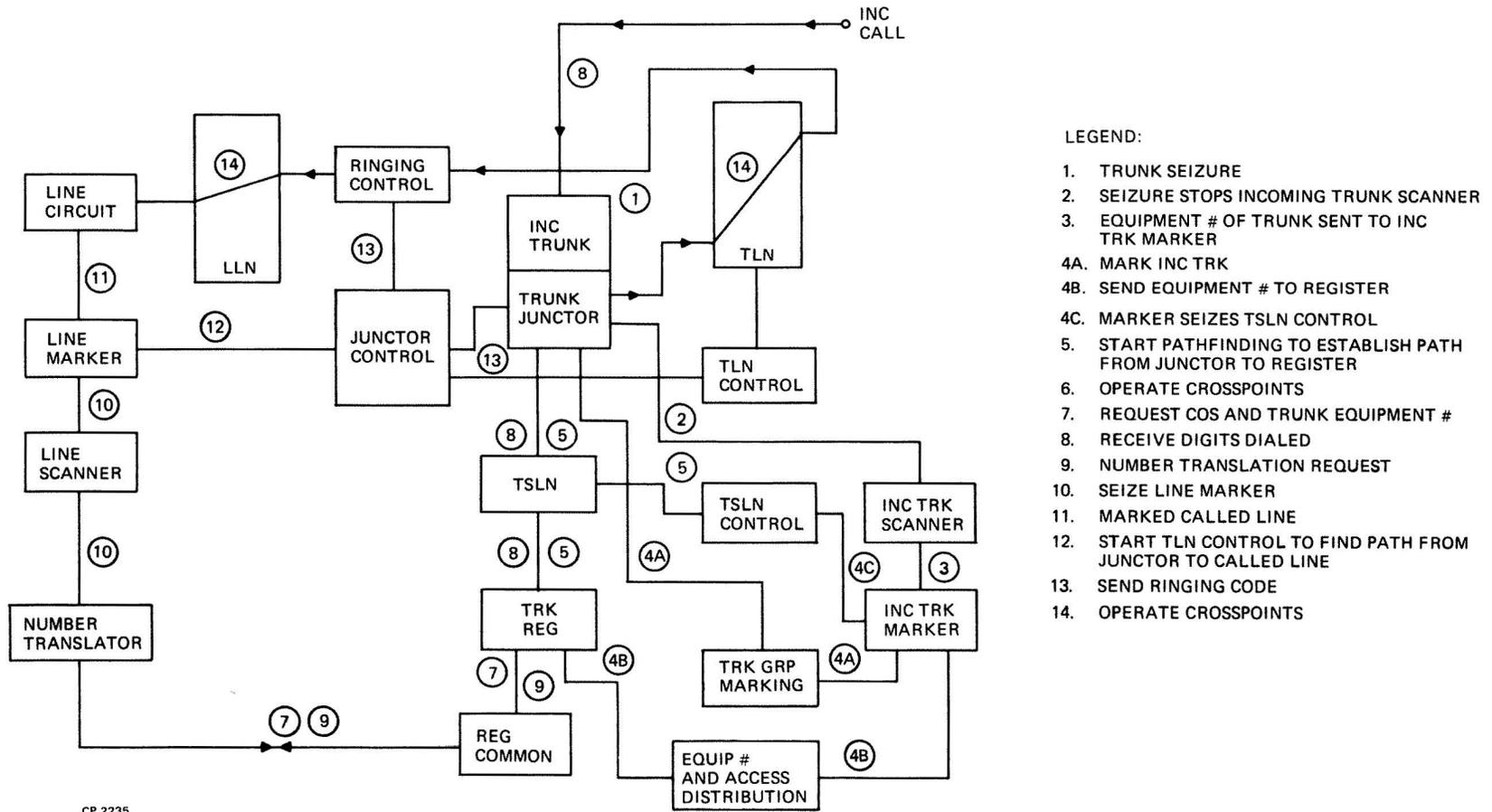
Figure 28. Trunk-to-Local Call, Functional Diagram
