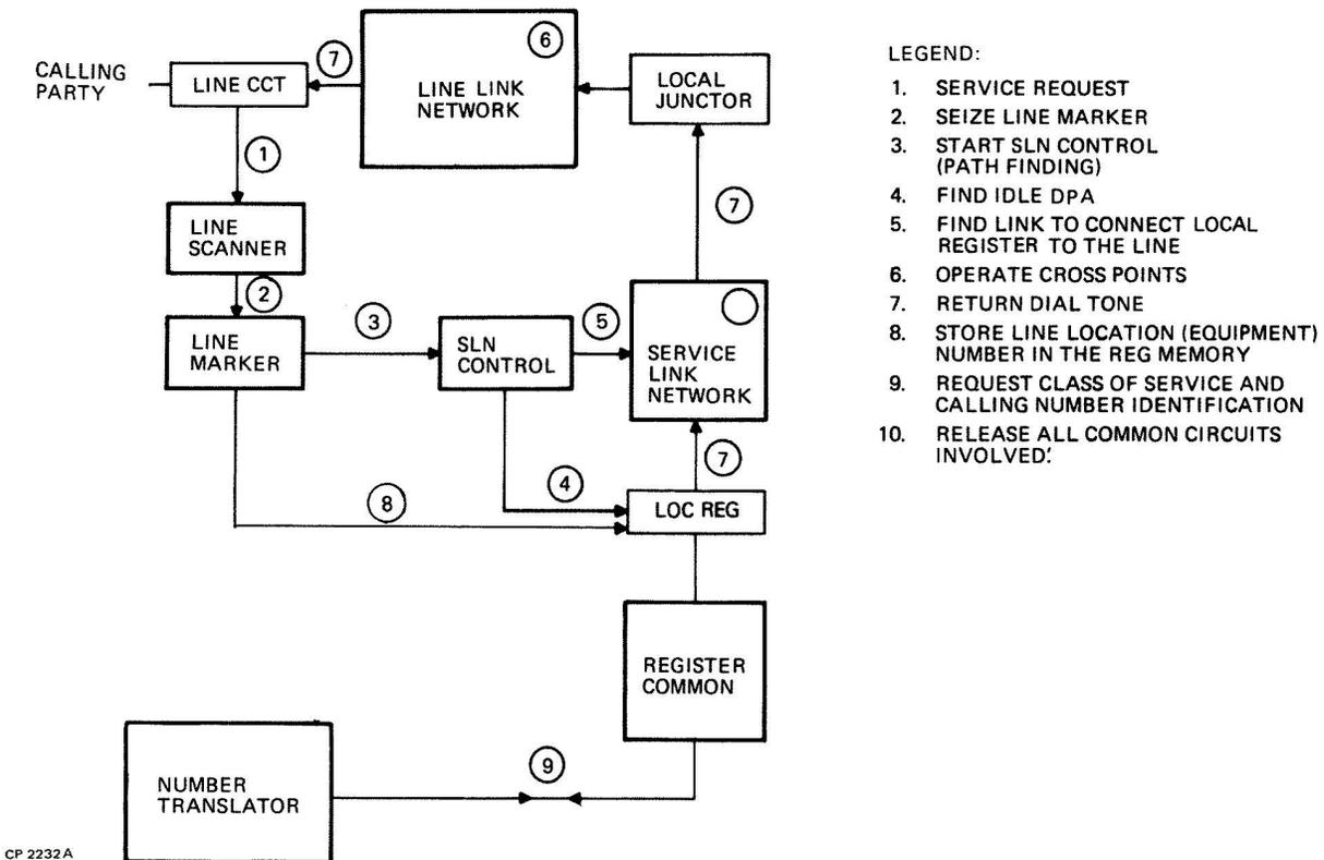
Figure 25. Dial-Tone Connection, Functional Diagram
