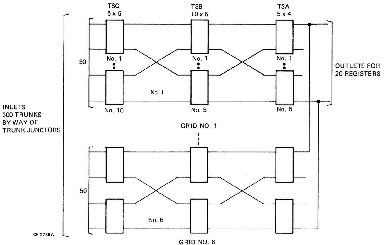
Figure 16. Trunk Service Link Network
