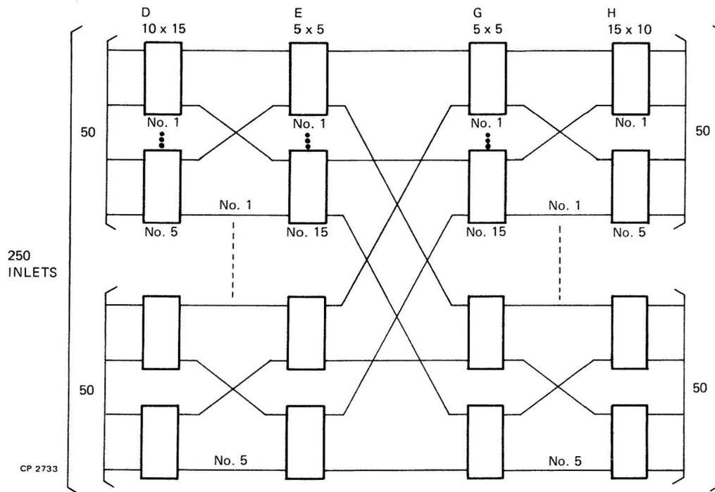
Figure 10. Four-Stage Trunk Link Network
