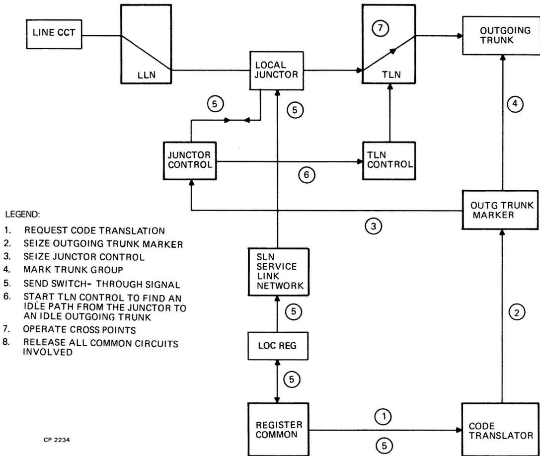
Figure 27. Termination of a Trunk Call, Functional Diagram
