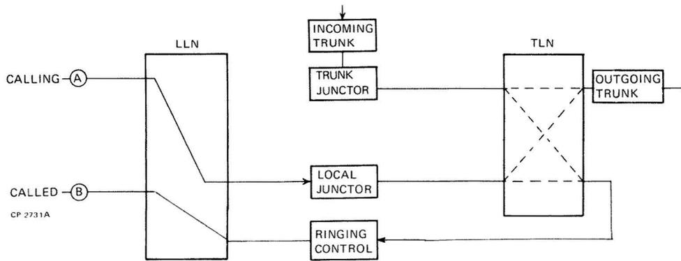
Figure 8. Transmission Switching Network
