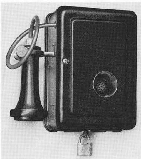
Fig. 1—The locked case, internally mounted transmitter, and heavy receiver cord are the external features that differentiate the 629A subscriber set from the usual type
