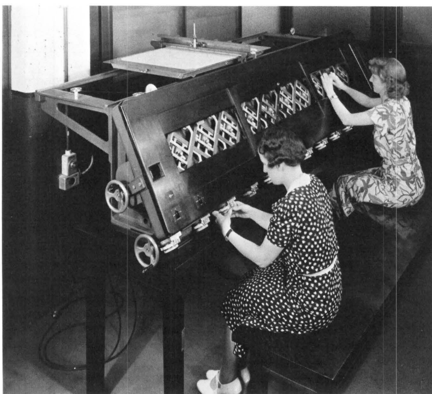
Fig. 1-18. The isograph, an invention of T. C. Fry, built in 1937 to locate complex roots of polynomials. At the top of the machine a pen plotted a curve, like a Nyquist diagram, from which one could deduce the number of zeros contained within a given circle in the complex plane.
