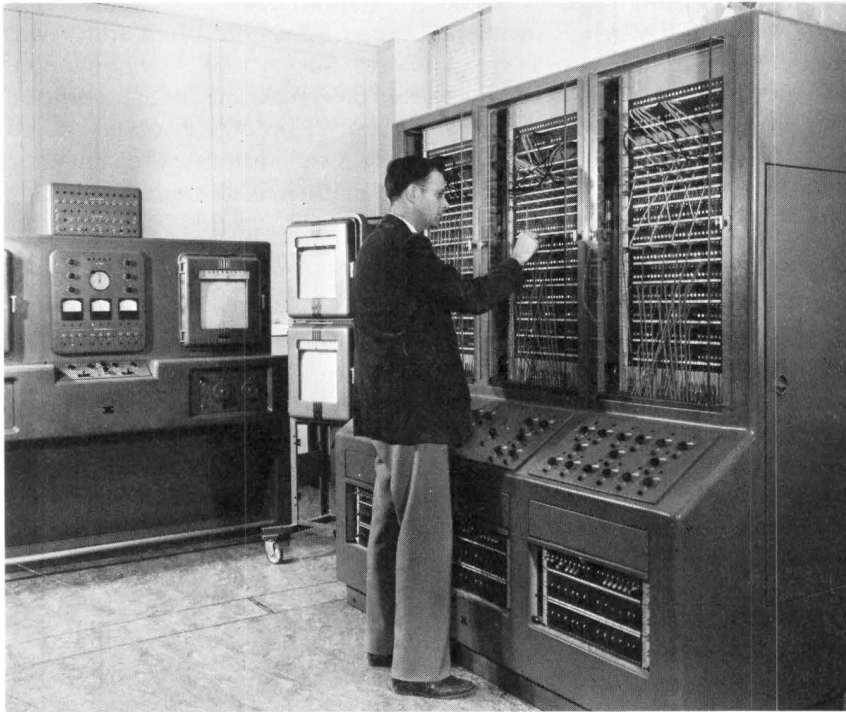
Fig. 9-1. R. W. Hamming setting up a problem on the general-purpose analog computer, Gypsy, which was designed by E. Lakatos and placed in service in 1949. Gypsy was relatively easy to change from problem to problem; output normally appeared on an electrically driven plotting board.
