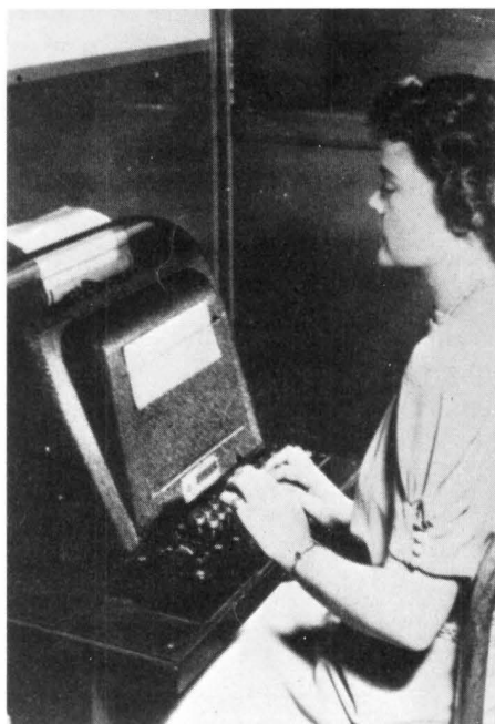
Fig. 9-3. One of three operator stations for the Model I, also known as the complex number computer. [Tropp, IEEE Spectrum 11 (1974): 70.]
