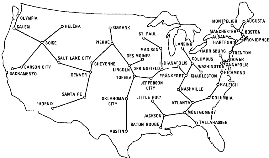
Fig. 1-12. "Minimal tree" for interconnecting 48 state capitals, using lines of the minimum total length, as required by tariff regulations. J. B. Kruskal and R. C. Prim developed efficient algorithms for finding minimal trees.
