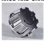
The Knob and Shaft Assembly is a replacement component for the Coin Return Lever on all coin telephone sets. It contains a slip clutch that prevents excessive torque from being applied to the coin return mechanism. It is used in locations where the Coin Return Lever is damaged by vandals.
