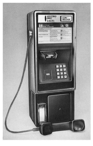
The Electronic Coin Public Telephone (ECPT) is a dialtone-first, microprocessor controlled public telephone that is equipped for touch-tone dialing. The 3A2 Coin Telephone utilizes advanced electronics to eliminate much of the electromechanical complexity found in the 1-type Coin Telephone Sets.
