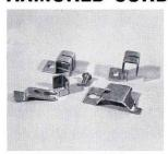
The Armored Cord Security Cable Retainer (Kit of Parts D181172) anchors the armored cord in the G3AM- and G3AN-type Handsets to the inside of any 1C- or 1D-type Coin Telephone Set. The retainer attaches to the pressed-on slug on the end of the stainless steel cable inside the armored cord.
