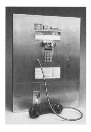
The 2C- or 2D-type Panel Coin Telephone is the "industry standard" for a panel-type coin public telephone. It is designed for flush- or corner-mounting and includes most of the features and options available with the 1C- or 1D-type Standard Coin Telephone respectively. Sets may be factory wired for dial-tone-first or coin-first operation. Transmission and signaling are equivalent to the 500-type telephone sets.
