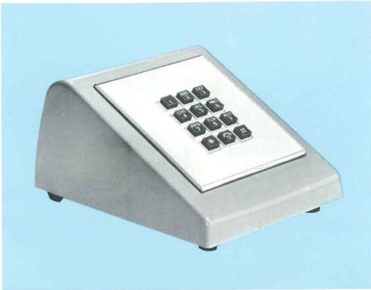
Stromberg-Carlson's 135 C3A TONE-DIAL pad allows you to give end-to-end signaling service even though the central office is only equipped for rotary-dial. It works this way: a computer access number, for example, is dialed in the usual manner on a rotary-dial telephone; once a circuit is established, the TONE-DIAL pad produces the tones required for information transfer. The pad can be used with a speaker-phone. Colors: page 13: white, beige, ivory, green, black, or gray.
