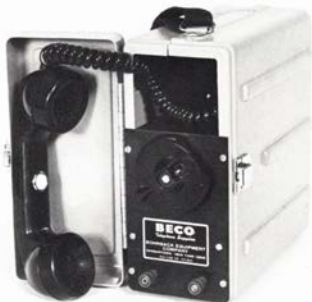
BECO MODEL 88A COVER OPEN HANDSET FITS IN COMPARTMENT WHEN CARRIED
