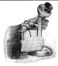
To inspect the hook switch, loosen the knurled nut at top of stem. You do this with your fingers: there are no mysterious "catches" or patent spring locks to monkey with.
