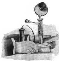
As soon as the nut is loose, the casing may be removed. Now you can see every working part and every wire, and yet every part is operative. There is not a sliding contact in the stand. Every connection is soldered.
