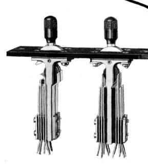
The Kellogg switchboard key assembly is a distinct engineering and mechanical achievement. The spring assemblies are rigidly mounted to a heavy T-shaped frame, firmly secured to a heavy brass escutcheon with baked enamel finish presenting a piece of apparatus smooth and accurate in operation, yet rigid and sturdy in construction.
