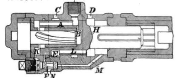
and passes to the passages A, and so to the rear end face of the piston H, thereby forcing it to the right. At the same time air passes by ports B to the hollow interior of the piston H and assists in propelling it. The incoming air also enters the passage
