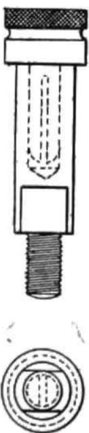
device to take the place of the usual nut secured on the end of the spigot to retain the wheel. The spigot is formed with a longitudinal hole extending for a substantial distance from its end and a split pin with a head is pushed into the hole and held therein by the spreading force of the split portion, which is
