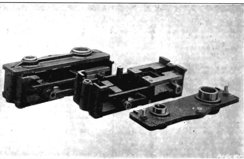
FIG. 5—BORING FIXTURE FOR LARGE AND SMALL ENDS OF CONNECTING RODS
