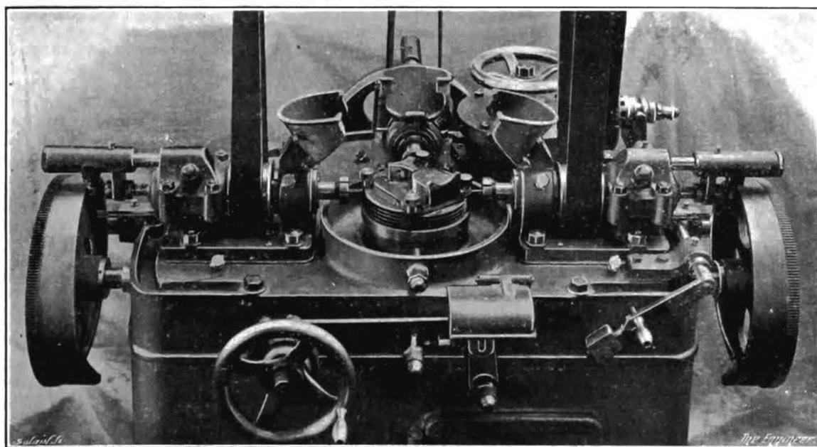
FIG. 1—THREE-SPINDLE MACHINE FOR MILLING CYLINDER HEADS FOR AERO-ENGINES
