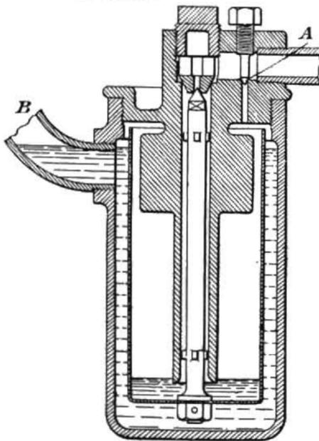
of a small leakage vent A. The inlet B is arranged below the lip of the bucket, and thus forms a seal between the air main and the leak A when the trap is full. The leak reduces the air pressure above the water in the trap, which then rises over the lip of the bucket and is discharged in the usual manner.—February 5th, 1920.
