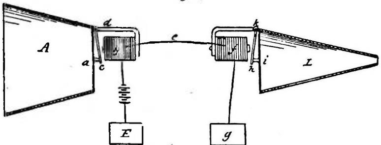
FIG. 10.—Figure 7 of Bell's patent.
