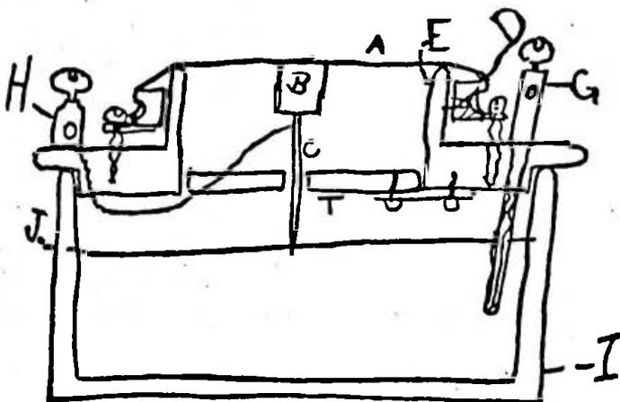
FIG. 11.—Watson's sketch of Bell's liquid transmitter.
