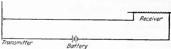
FIG. 5.—Principles of Reis' make and break telephone.
