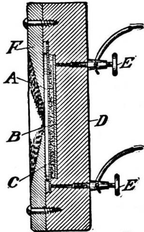
FIG. 20.—Hunnings' granular carbon transmitter.
