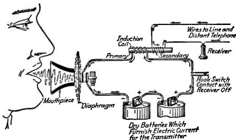
FIG. 22.—Talking circuit of a local battery telephone.
