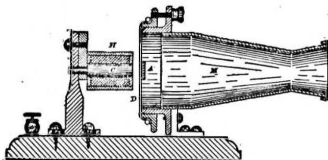
FIG. 13.—Bell's Centennial magneto transmitter.
