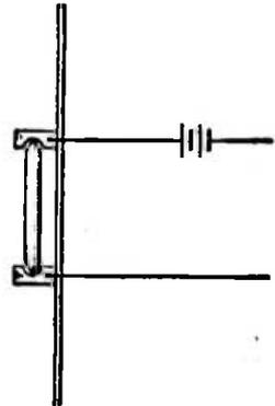
FIG. 19.—Hughes' carbon microphone.
