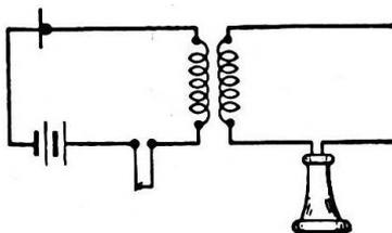
FIG. 23.—Talking circuit of local battery telephone.
