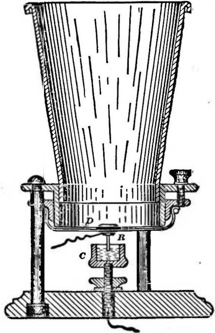
FIG. 12.—Bell's Centennial liquid transmitter.
