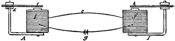
FIG. 9.—Figure 5 of Bell's patent.
