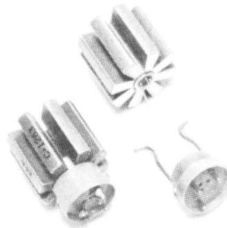
Fig. 17-5. The 24-type silicon transistor used in the N2 line amplifier with its heat dissipating mounting socket.
