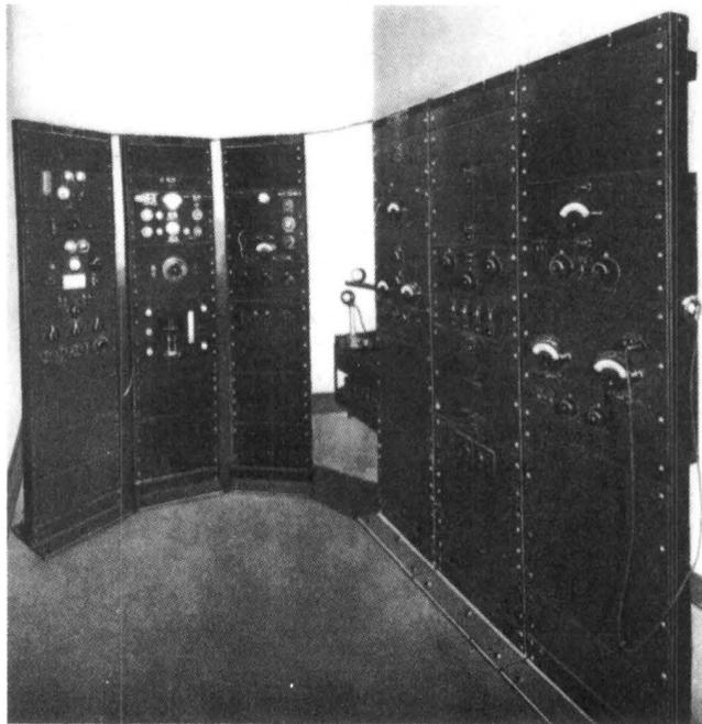
Fig. 21-3. Master Reference System for Telephone Transmission with associated calibration apparatus. This system was adopted as an international standard in 1926.
