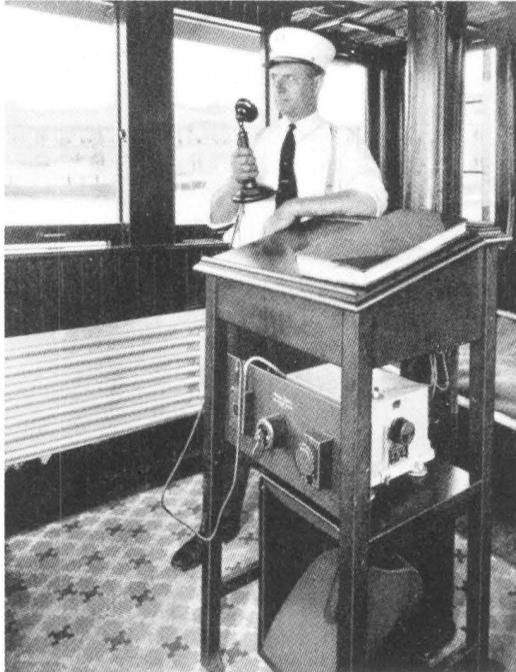
Fig. 14-2. Coastal and harbor radio equipment on a fireboat in New York harbor, 1930. The receiver is on the shelf above a loudspeaker on the deck.
