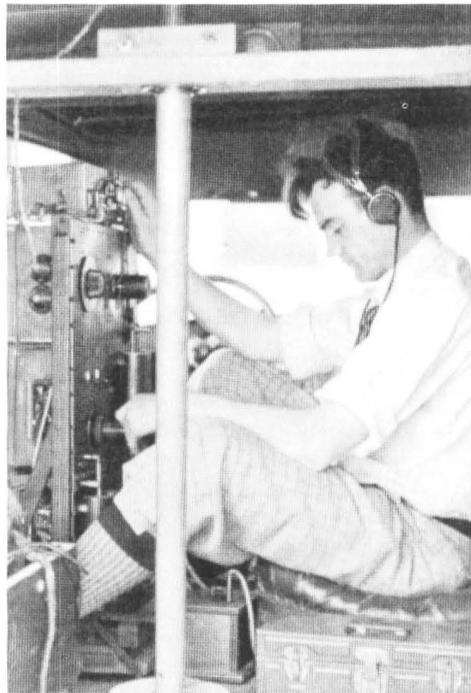
Fig. 7-4. Automobile-mounted receiving equipment for measuring the strength of ultrashortwave fields during overland traverses.
