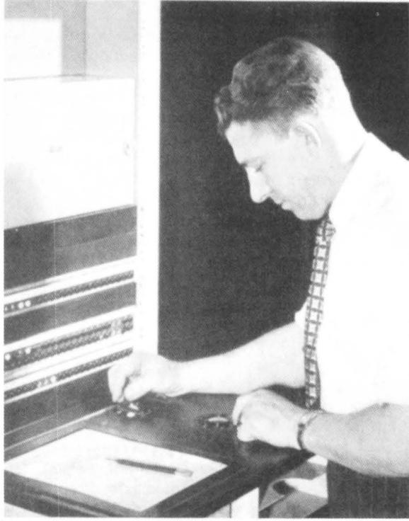
Fig. 23-4. Recording troubles indicated by lamps under a log sheet at an L1 coaxial system maintenance center, 1950.
