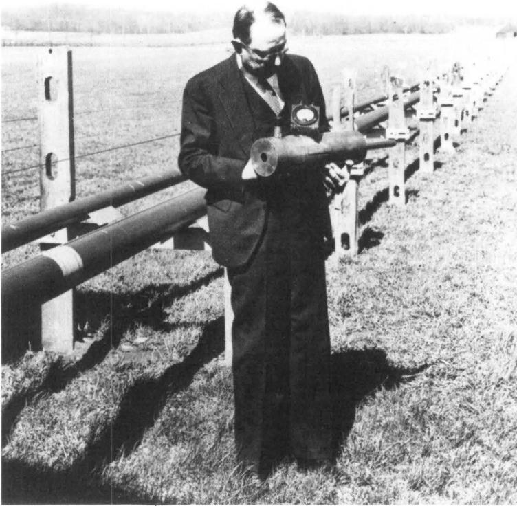
Fig. 7-14. G. C. Southworth in front of the circular-electric-mode waveguide transmission line built at Holmdel, New Jersey in 1935. Southworth is holding one of the resonant chambers used for tests of waveguide transmission.
