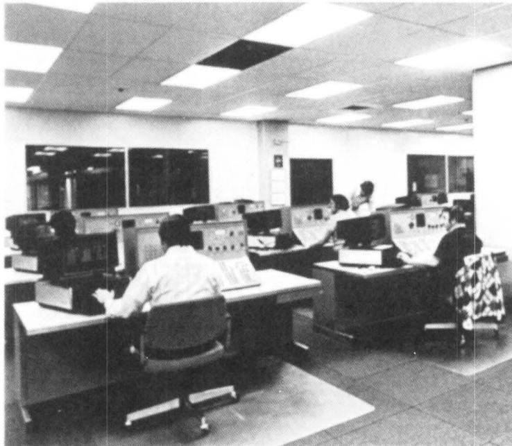
Fig. 23-14. The trunk operations center for the 4ESS switch showing CMS1A CRT terminals at 51A test positions.
