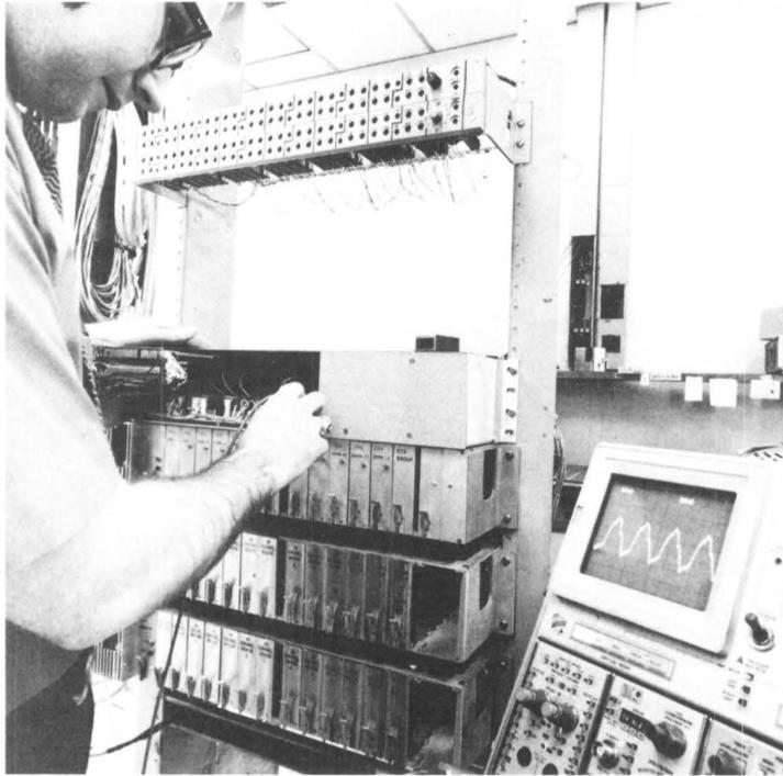
Fig. 15-11. A laboratory prototype A6 channel bank assembly. The patch panel is at the top of the frame.
