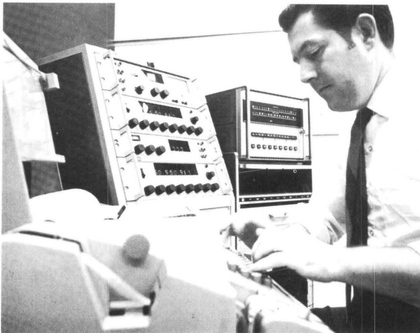
Fig. 10-23. Remotely controlled programmable Type 90 oscillator and detector for the L5 transmission-surveillance auxiliary.
