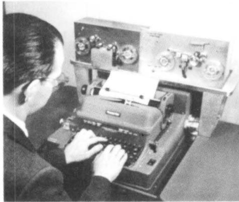
Fig. 22-15. Experimental data transmission over telephone channels, 1957. (a) Transmission from a prerecorded magnetic tape via a data subset modem. (b) Electric typewriter and experimental equipment for use of magnetic tapes to store data for transmission.
