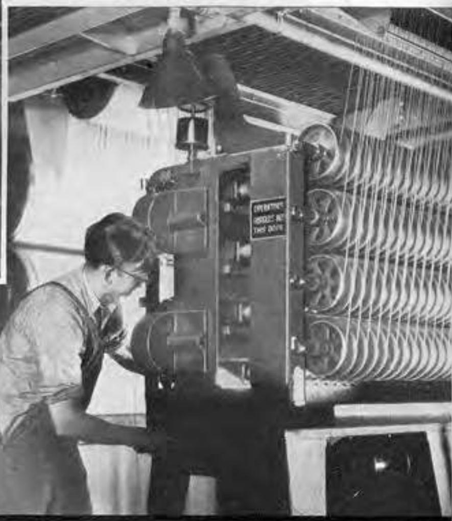
Makes paper insulation on 60 wires at once.
