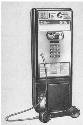
The 1D-type Standard Coin Telephone is the "industry standard" for a single coin slot public telephone. It may be equipped for either rotary or touch-tone dialing. It is an exceptionally high reliability, high security device and, with available options, may be used in most adverse environments. Operation is in the dial-tone-first mode which permits placing of emergency or other selected calls without a coin deposit. Transmission and signaling is equivalent to the 500-type telephone sets.
