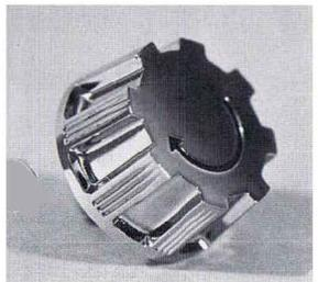
The Knob and Shaft Assembly is a replacement component for the Coin Return Lever on all coin telephone sets. It contains a slip clutch that prevents excessive torque from being applied to the coin return mechanism. It is used in locations where the Coin Return Lever is damaged by vandals.
