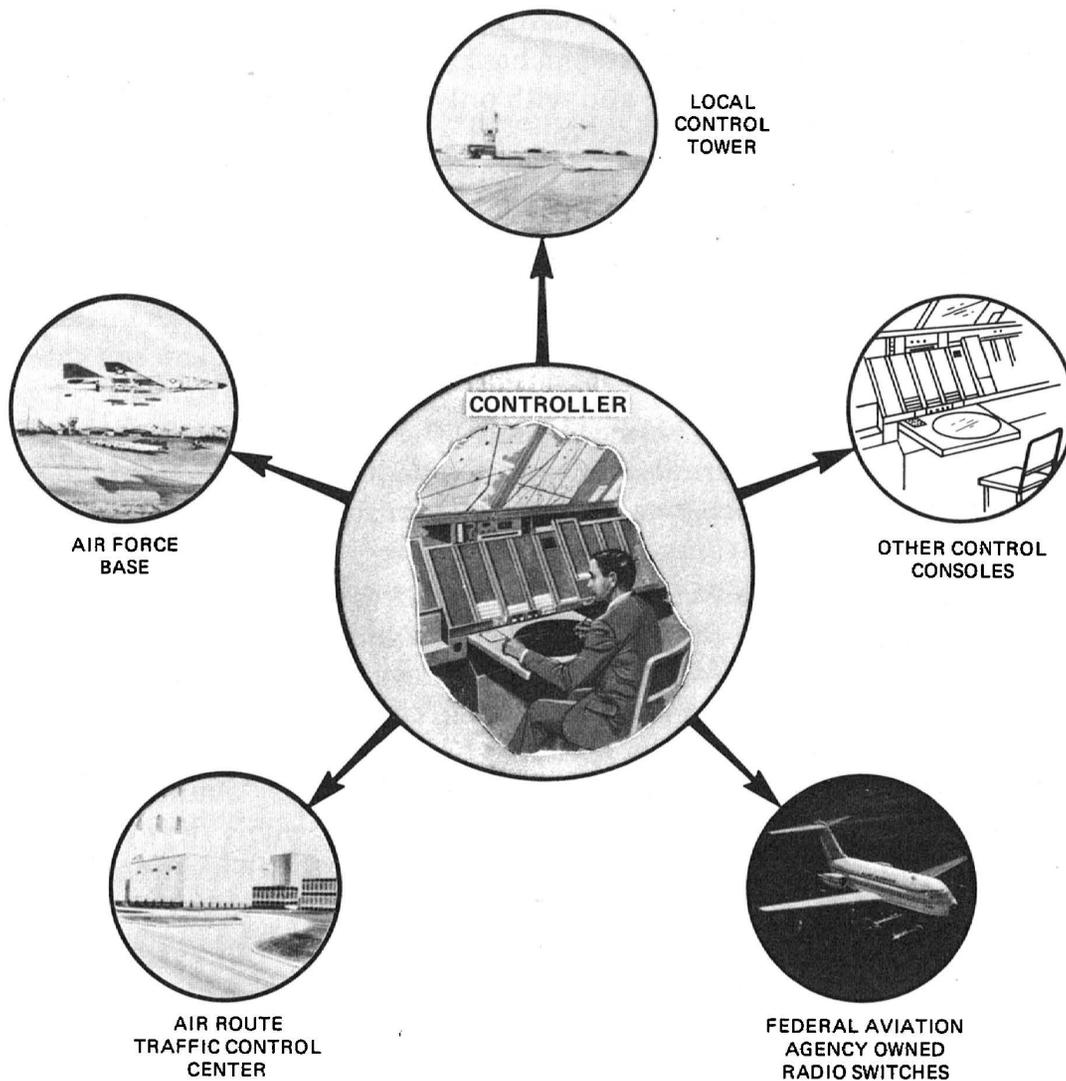
Fig. 12-17. Air route traffic control voice-communications system.
