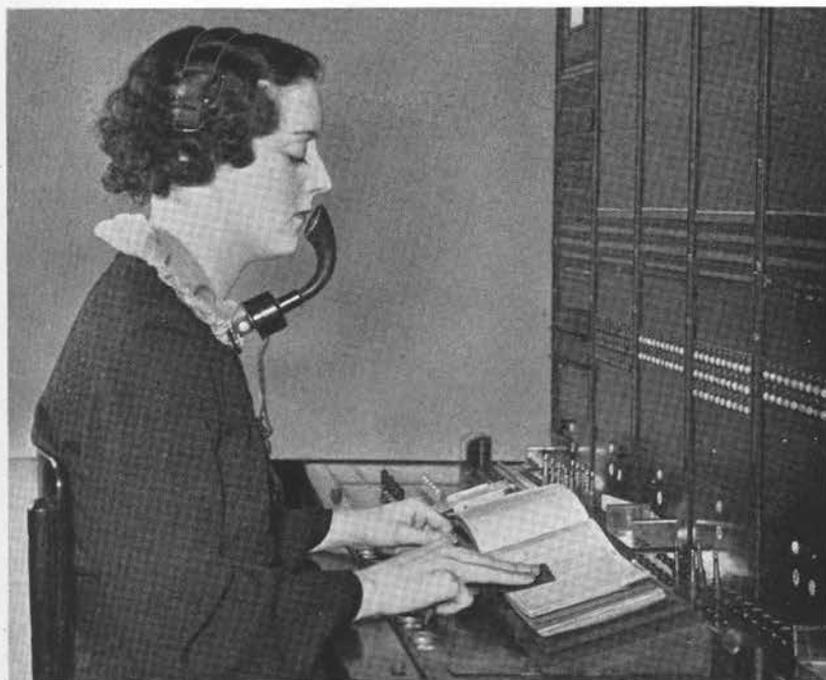
*A shorter mouthpiece has recently been developed for operators' transmitters, primarily for use where records have to be consulted frequently, such as at information and intercepting positions. An improvement in vision results and this in turn provides more uniform transmission since there is less need for an operator to turn away from her mouthpiece.*
