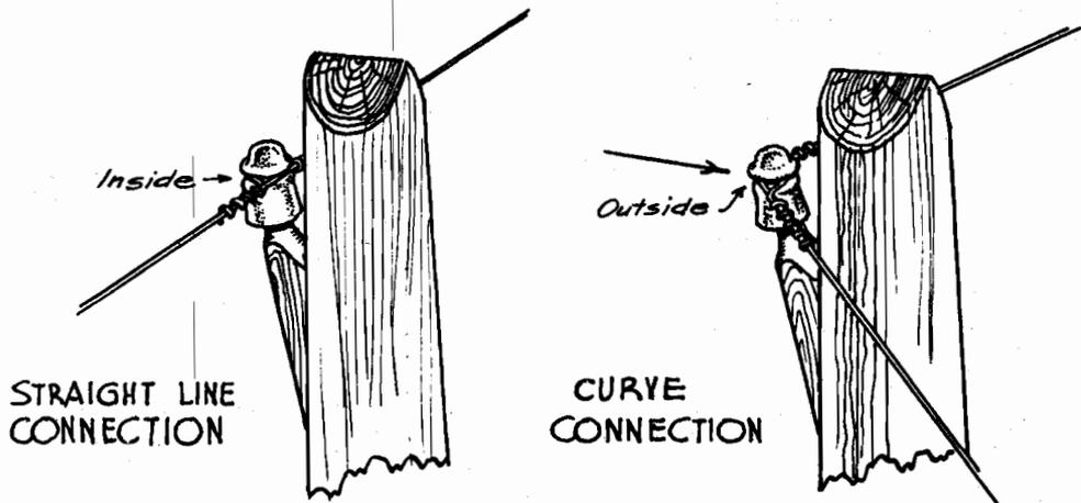
In crossarm line construction the wire should be fastened as follows:
