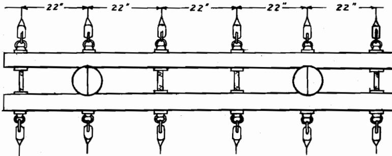
PIN SPACING FOR SPANS UP TO 500 FEET
