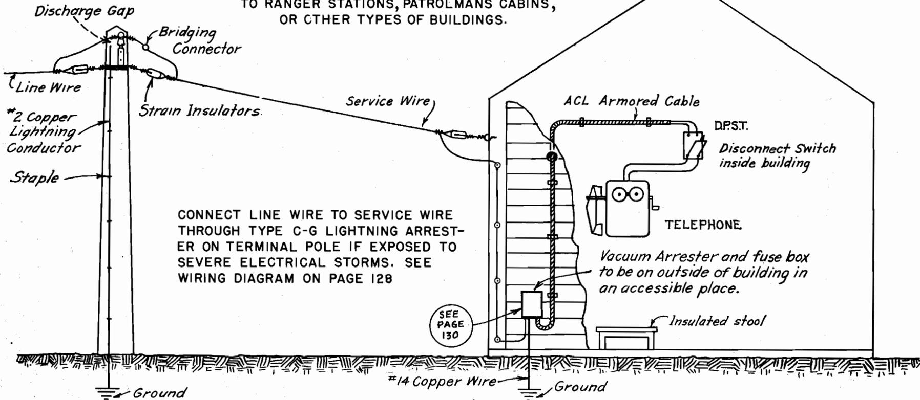
CONNECT LINE WIRE TO SERVICE WIRE THROUGH TYPE C-G LIGHTNING ARRESTER ON TERMINAL POLE IF EXPOSED TO SEVERE ELECTRICAL STORMS. SEE WIRING DIAGRAM ON PAGE 128
