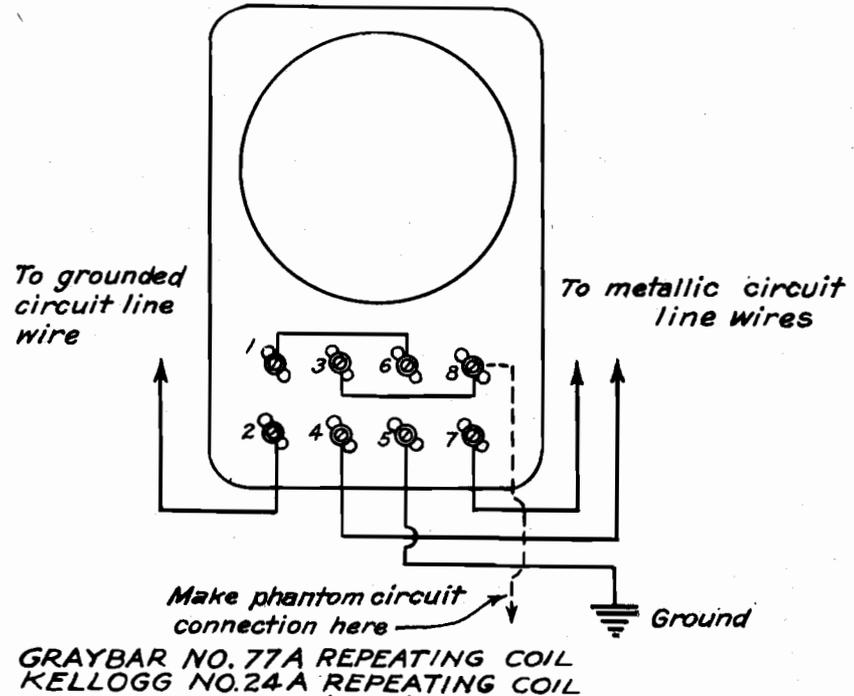
If coils are mounted outside, (on pole or elsewhere) vacuum protectors are to be used, two on the metallic circuit side and one on the grounded circuit side
