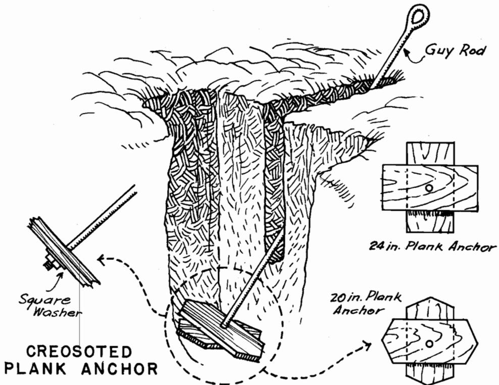
The standard size for anchor guy rods is  $5/8"$  x 6' except in moist or loose soil where an 8 foot rod is necessary to obtain sufficient purchase. Either galvanized iron or copper-covered rods may be used. Unless the thimble-eye rod is used, a guy thimble must be installed in the eye of the rod as a protection for the guy strand.
