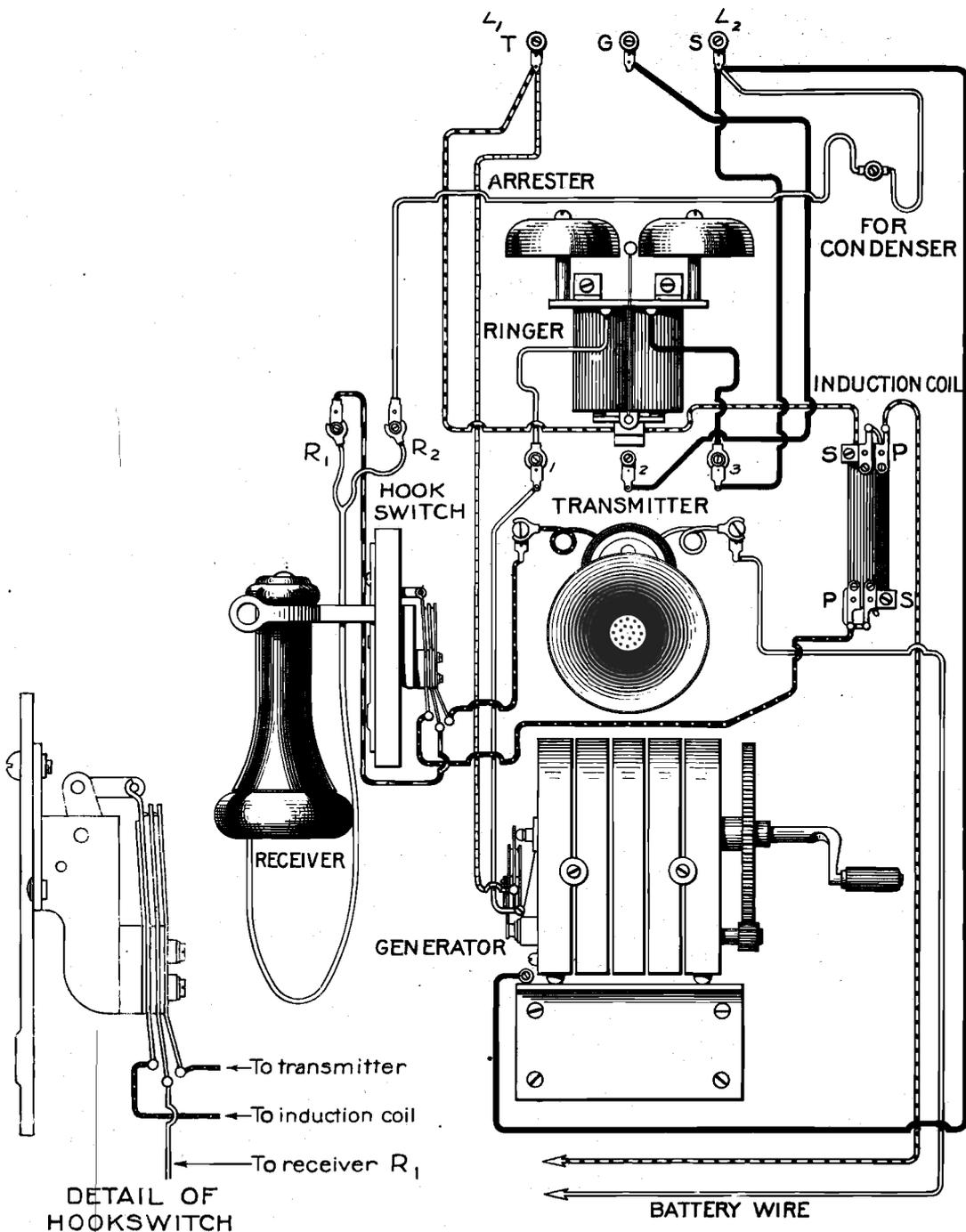
WIRING DIAGRAM OF KELLOGG TELEPHONE
