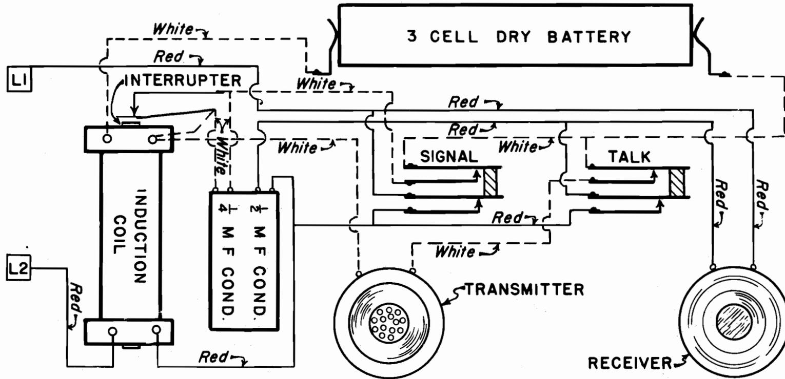
WIRING DIAGRAM OF
