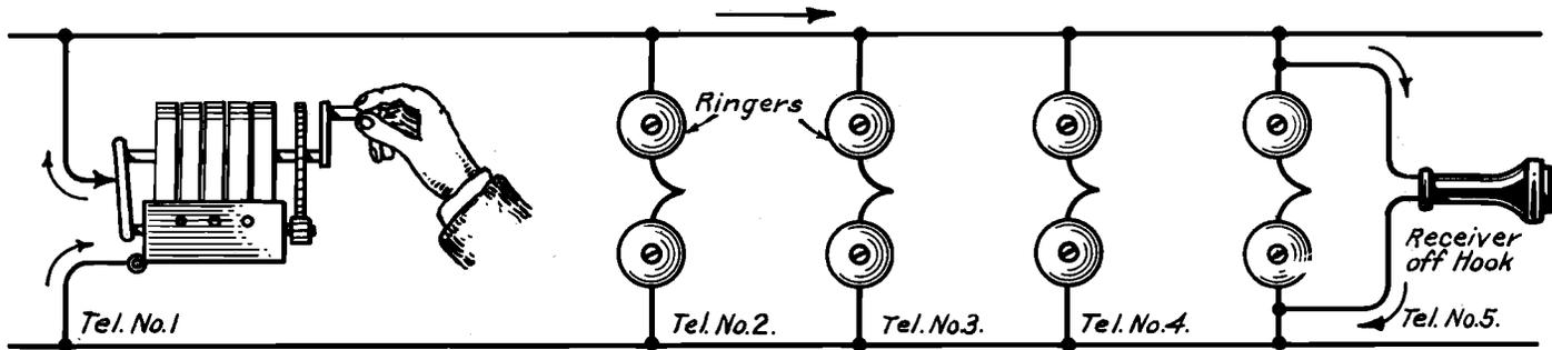
IMPOSSIBLE TO RING OTHER TELEPHONES, DUE TO RECEIVER OFF HOOK AT TELEPHONE NO. 5, ALLOWING MOST OF THE RINGING CURRENT TO PASS, INDICATED BY ARROWS
