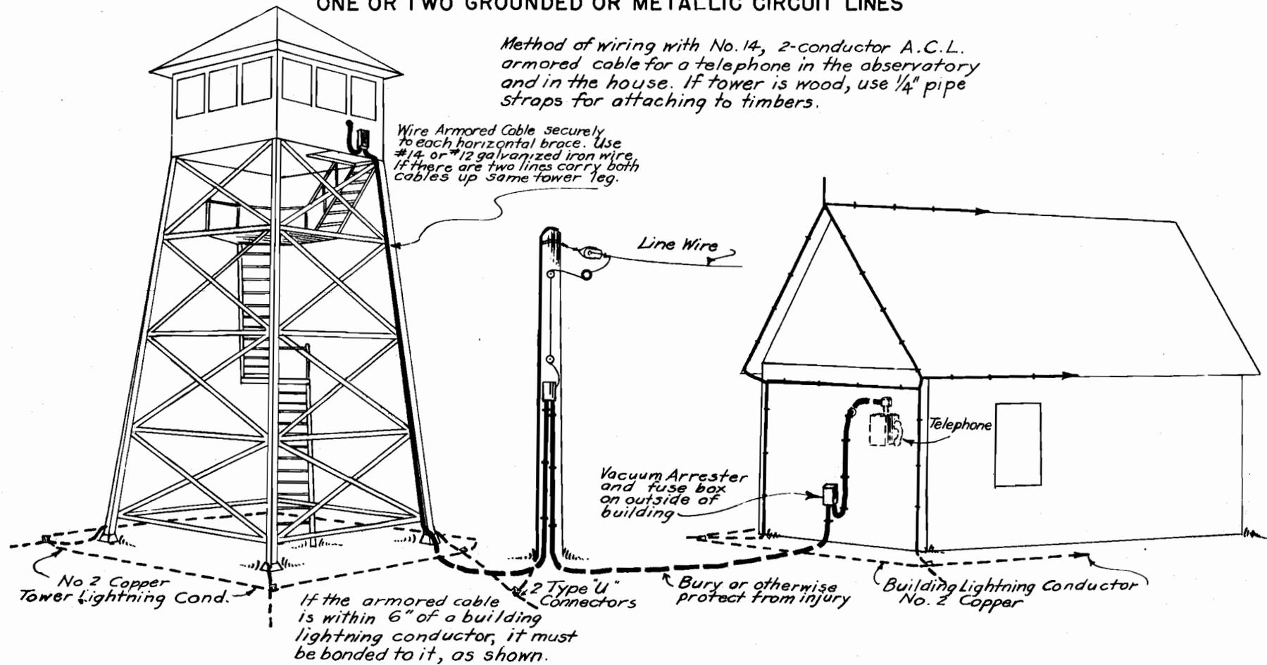
*Method of wiring with No. 14, 2-conductor A.C.L. armored cable for a telephone in the observatory and in the house. If tower is wood, use 1/4" pipe straps for attaching to timbers.*
