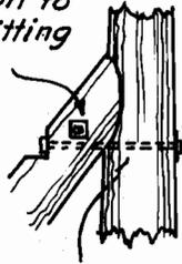
Crossarm bolt to pass through brace at this point.
