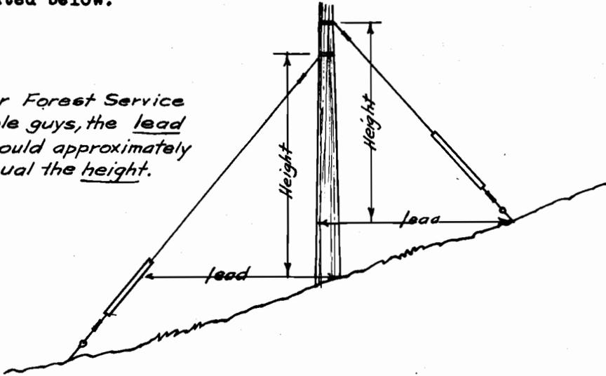
Guy wires should bisect the angle of strain. In order to lessen the strain, it is preferable to use a two-pole corner rather than make the curve on one pole.
