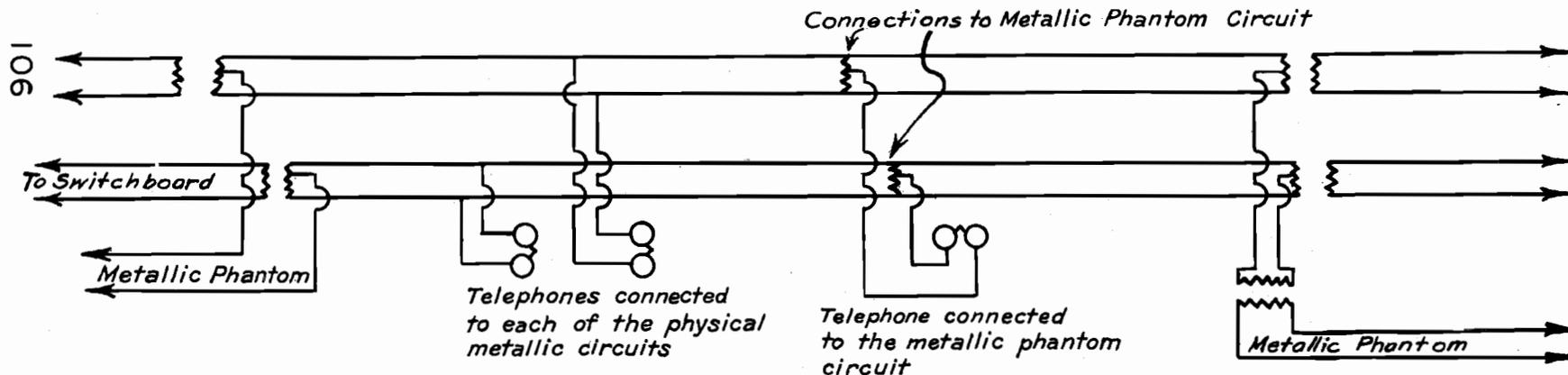
**SCHMATIC DIAGRAM SHOWING CONNECTIONS FOR A METALLIC PHANTOM CIRCUIT**
