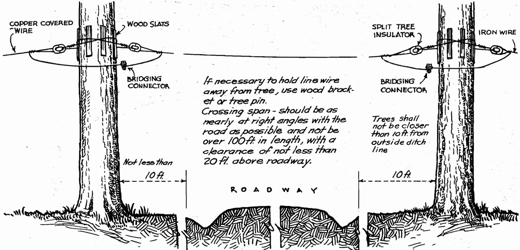
*If necessary to hold line wire away from tree, use wood bracket or tree pin.*
