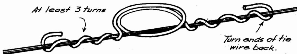
If the modified horseshoe tie is used where there is no change in grade, one end should be wrapped as shown for "under tie" and the other as shown for "over tie."
