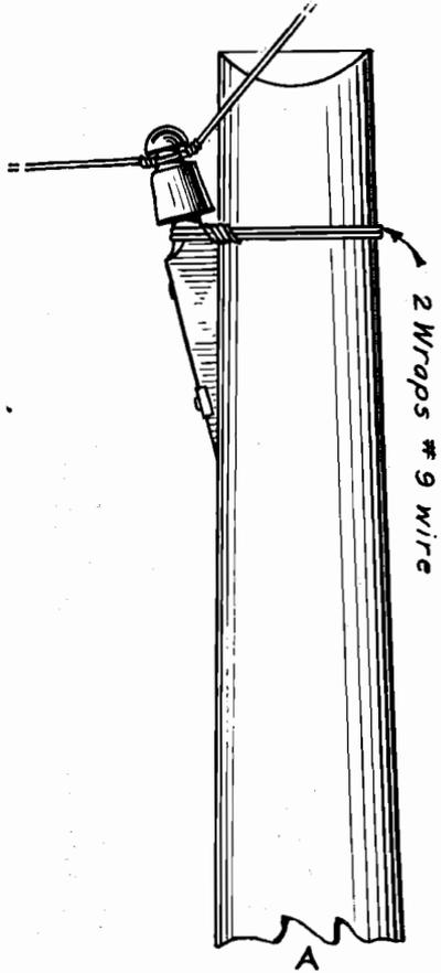
Method of attaching wire where pull away from pole is unavoidable. Method "B" is preferable.
