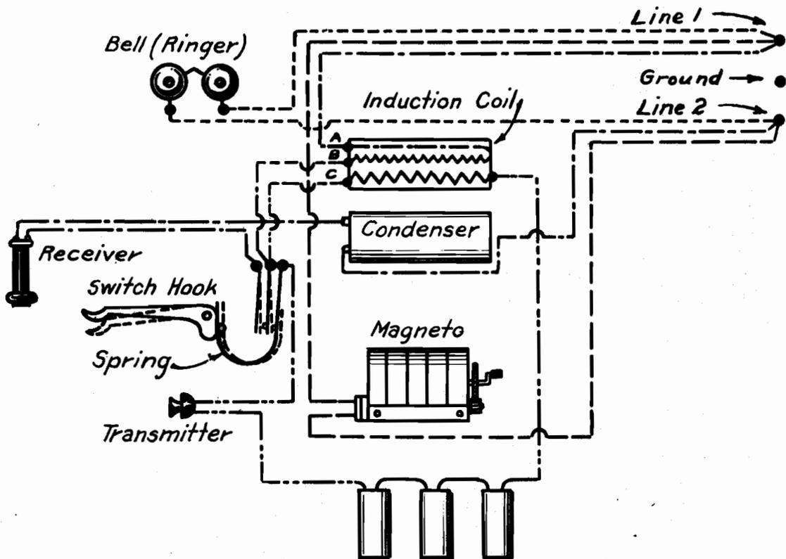
*In many Telephones "B" and "C" are connected together at the induction coil, with only one wire extending to the switch hook.*
