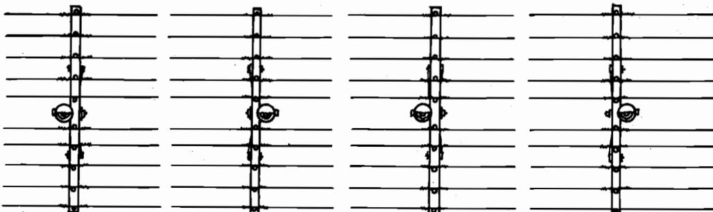
At single pole corners, face the poles so that the crossarms will bisect the angle and will be on the face of the pole away from the longer straight section of the line. Crossarms on the poles adjacent to the corner shall face toward the corner pole.
