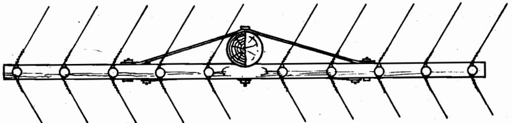
4. On transposition poles and on poles adjacent to transposition poles so that the pull will be against the insulator.
