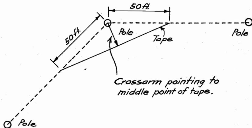
At two-pole corners, face the poles so that the crossarms will bisect the angle at each pole and so that the crossarms will be on the pole away from the adjacent straight section of line. Crossarms on the poles adjacent to the corner shall face toward the corner pole.
