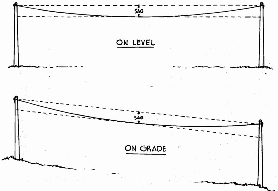
Correct sag is extremely important. Two methods are commonly used to determine the proper amount of sag in a span. One is the sighting method by the use of a sag gauge and the other is the oscillation method. In obtaining the proper sag by either method, proceed as follows:
