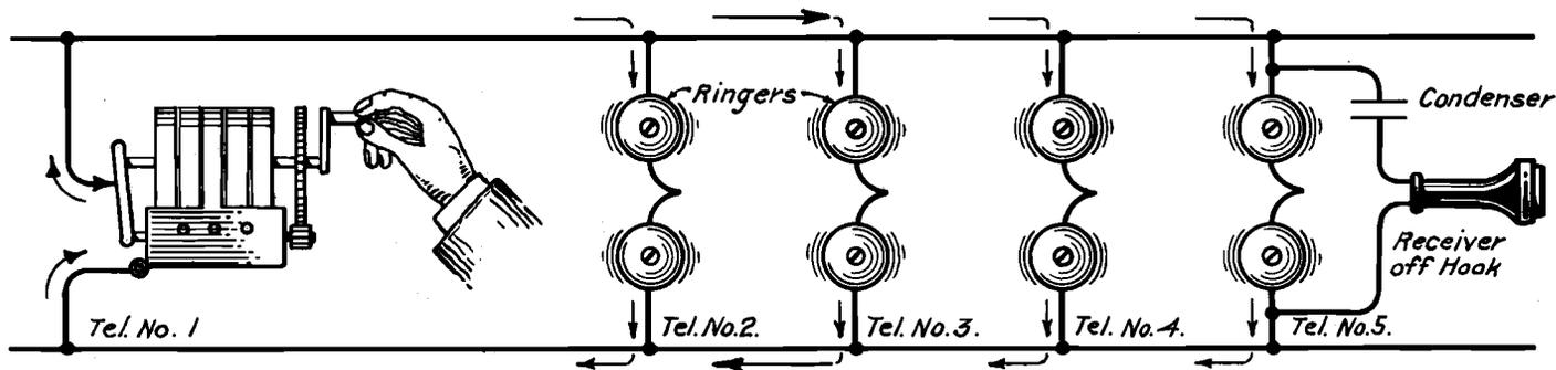
CONDENSER IN CIRCUIT WITH RECEIVER PREVENTS RINGING CURRENT GOING THROUGH RECEIVER, AND RINGERS ARE ALL FASILY RUNG
