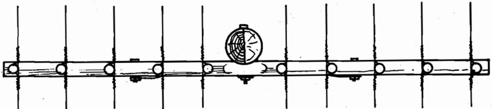
2. On straight sections exposed to heavy cross winds, on the side of the insulator facing the prevailing storm wind.
