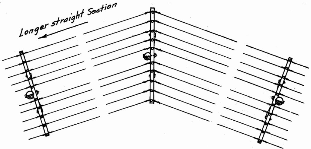
Note: A crossarm bisects the angle in the line when it points to the mid-point of a tape line stretched between two points laid off a convenient distance (50 feet, for example) along the lead from the corner pole.
