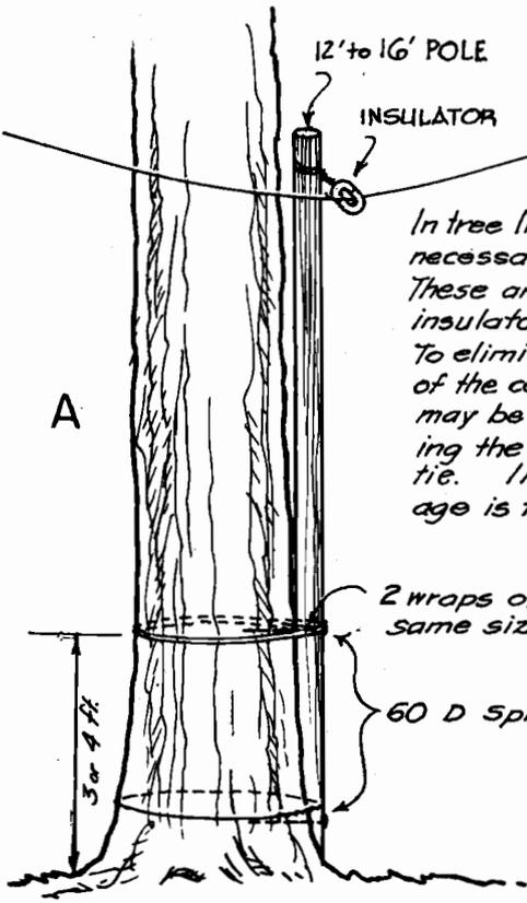
In tree line construction it is often necessary to tie to a large tree. These are often so rigid that an insulator pulls off. To eliminate this trouble, either of the construction methods shown may be used. Each avoids climbing the tree and gives a springy tie. Insulator and wire breakage is thereby reduced.
