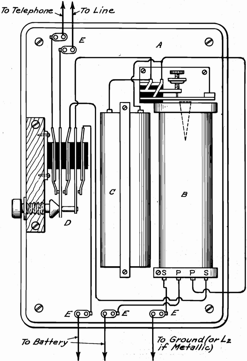
WIRING DIAGRAM FOR HOWLER SIGNAL SET
