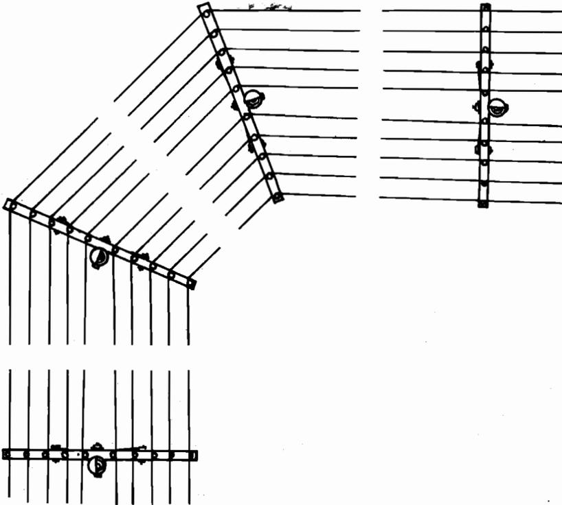
At open wire dead-ends, set poles with the face away from the last span. Set the pole next to the dead-end pole with the face toward the last span.
