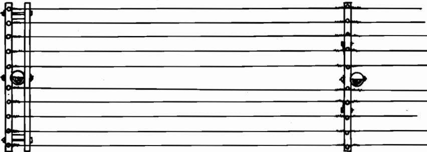
At long spans, face the poles supporting the long span away from the long span.
