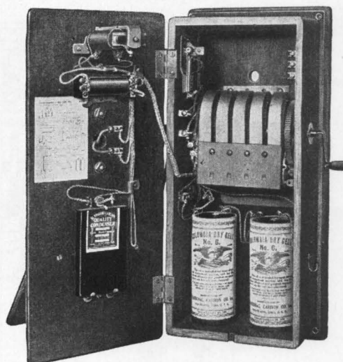
Open View of No. 896 Telephone
