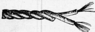
FIG. 252.—A twisted pair of insulated wires, forming two sides of a single circuit, as in telephone cables.
