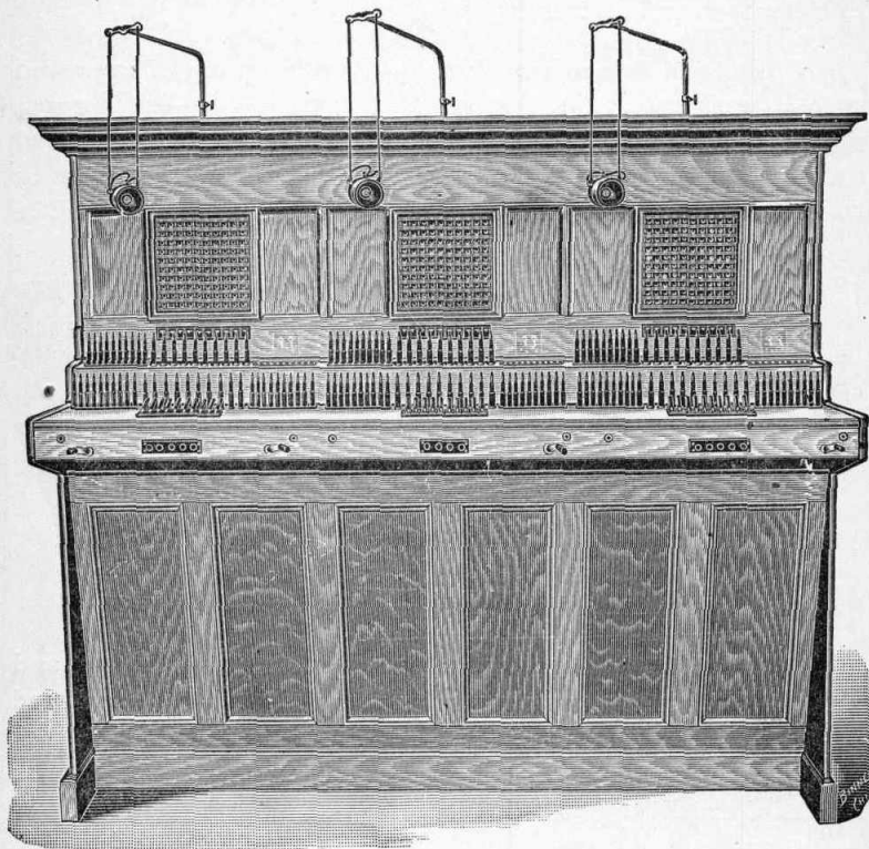
FIG. 139.—A 300-drop switchboard of the Western Telephone Construction Co., equipped with the type of drop-jacks shown in the last figure.
