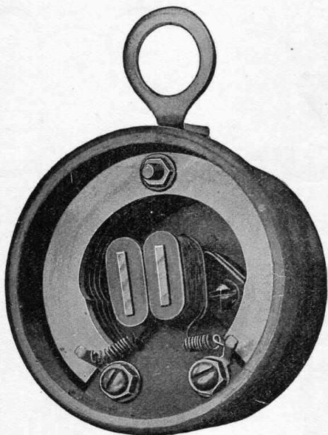
FIG. 59.—Interior view of a typical "watchcase" receiver.
