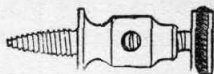
FIG. 4.—One form of binding post. The screw at its end is intended for contact with the electrical conductor, and the line wire is inserted in the hole through the centre, where it is held tight by the thumb screw.
