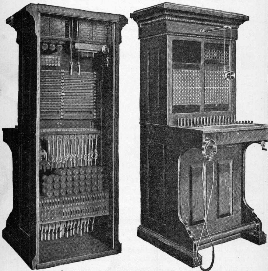
FIGS. 148a-148b.—Rear and front view of a switchboard using incandescent electric lamp signals.
