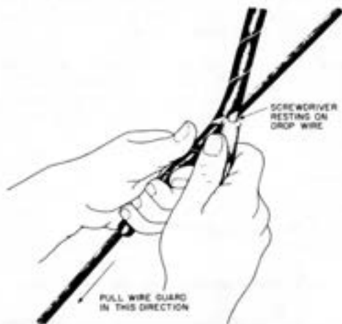
Fig. 3—Placing P Wire Guard Screwdriver Method
