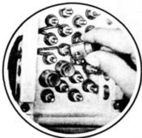
Fig. 18—Installing Binding Post Caps
