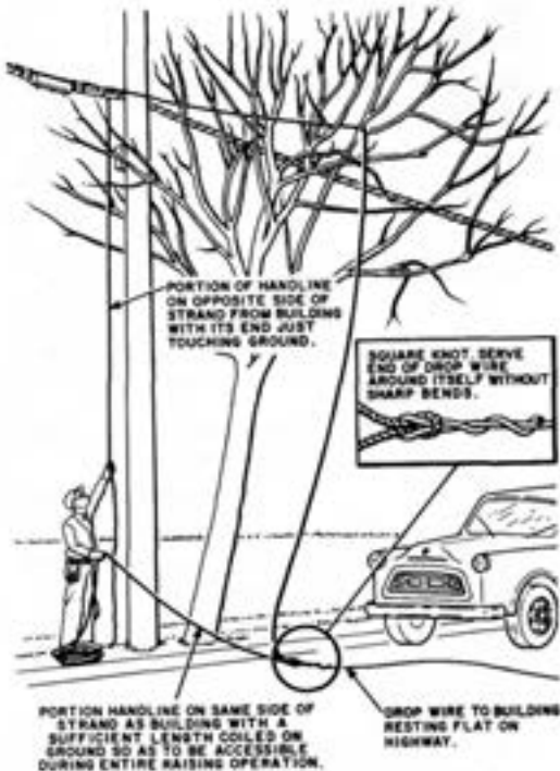
Fig. 7—Drop Wire Tied to Handline
