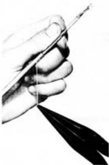
Fig. 7—Stripping SK Station Wire
