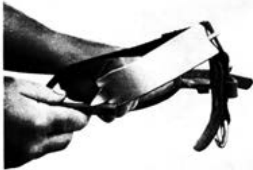
Fig. 19—Removing Burrs From Bottom Cutting Edge
