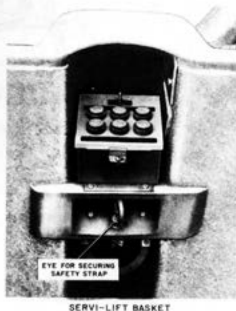
Fig. 9—Location of Eyes for Securing Safety Strap in Baskets of SKYWORKER and SERVI-LIFT Aerial Lifts
