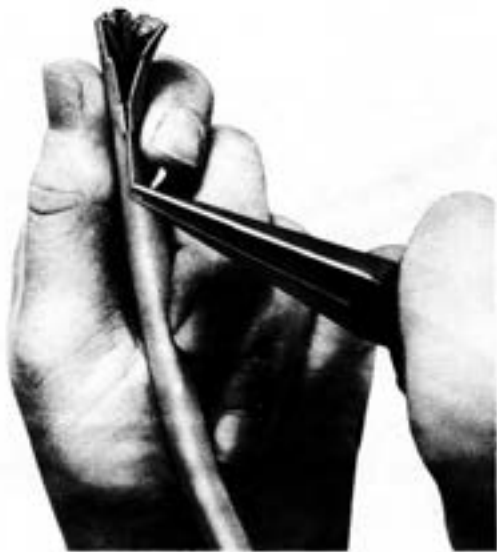
Fig. 6—Stripping D Inside Wiring Cable or G and H Station Wire (With Jacket-Slitting Cord)
