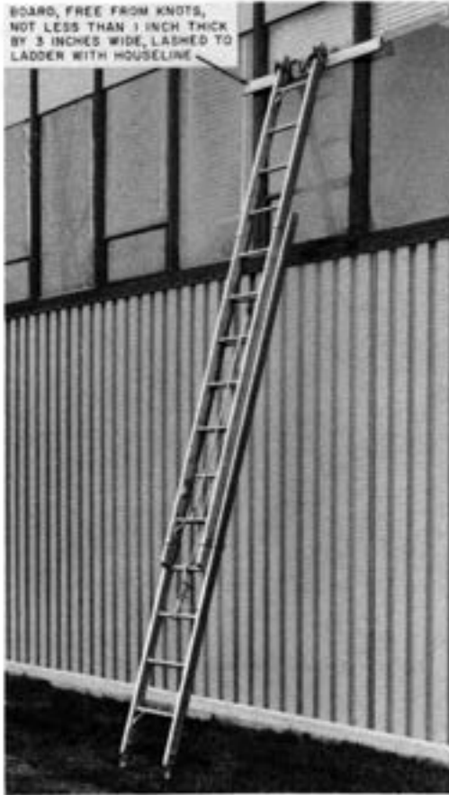
Fig. 16—Ladder Placed in Front of Window
