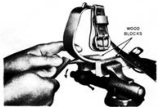
Fig. 21—Using Vise for Honing Gaff
