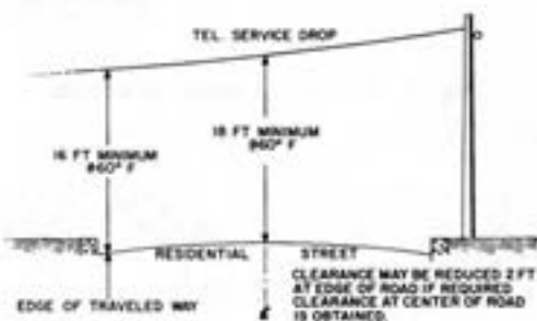
Fig. 3—Service Drop Over Residential Street
