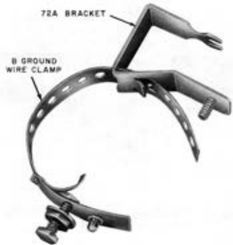
Fig. 35—B Station Ground Clamp Through Slots in 72A Bracket
