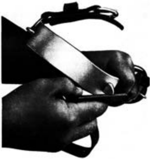
Fig. 18—Removing Burrs From Top Cutting Edge
