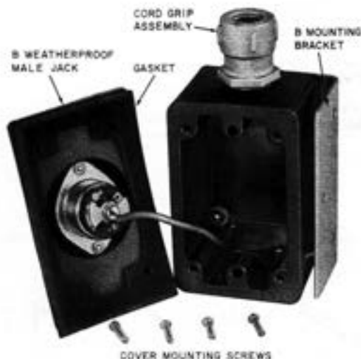
Fig. 9—B Weatherproof Male Jack on B Outlet Box Showing Ground Lead Connected to B Mounting Bracket
