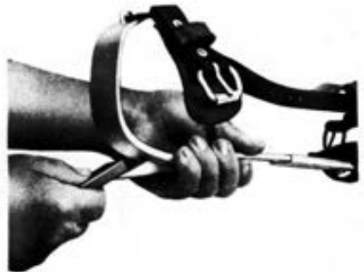
Fig. 20—Honing Inner Surface
