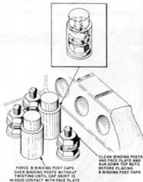
Fig. 28—Placing B Binding Post Caps
