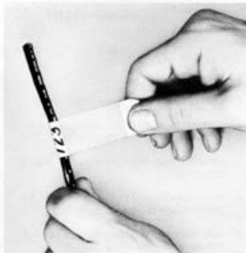
Fig. 1—♦Placing Self-Laminating Label♦
