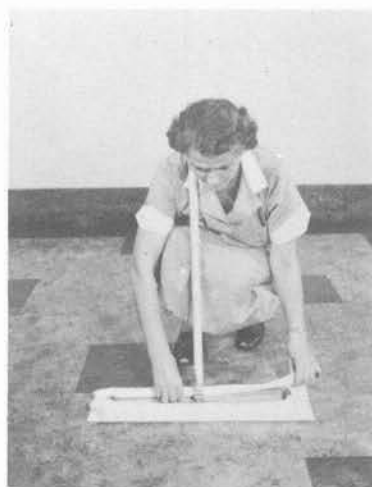
Fig. 4 – To remove cloth, pull from under lip at center and with side motion disengage cloth from boot. Turn tool around and remove from opposite side. Turn cloth over and reattach. To turn inside out, detach, spread cloth with soiled side down, grasp at center, lift to fold with clean side out. Reattach. Wipe up any soil dropped on floor.
