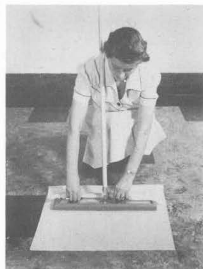
Fig. 2 – Rest handle on shoulder. With both hands free, tuck near edge of cloth under lip of the boot. Outer sides of cloth pass through slot in each corner of boot to overlap tool on each side. Tuck cloth well into slots in corners of boot.
