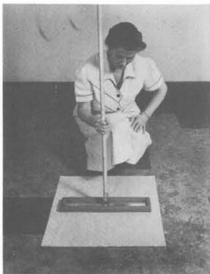
Fig. 1 – Spread cloth out on floor or other suitable flat surface, a little to one side. Grasp tool by handle and place it in center of cloth.
