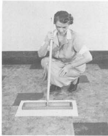
Fig. 1 – Fold cloth at center. Spread on floor or other suitable flat surface. Place tool in center of folded cloth.
