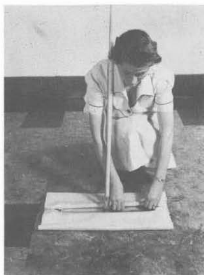
Fig. 3 – Without changing position, grasp handle and turn tool 180 degrees. Attach this edge of cloth in same manner. A loop of cloth is thus formed under tool.
