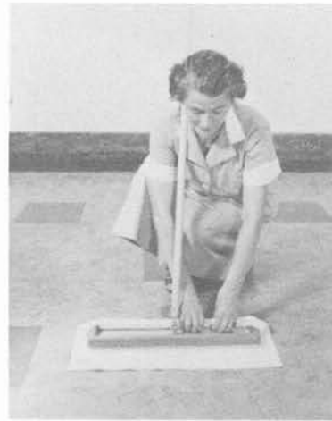
Fig. 2 – Rest handle on shoulder. Tuck near edge of cloth under lip of boot. Turn tool around and attach opposite side. Tuck cloth well into slot in each corner of boot.
