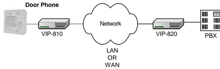
In this example, the VIP-810 and VIP-820 are connected to the data network to extend the station port to a telephone at a remote location. This could be installed where network access is available, but not telephone wiring.
