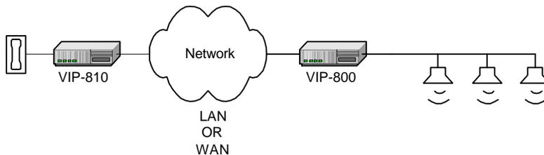
In this example, the VIP-810 and VIP-820 are connected to the data network to extend the station port to a remote Door Phone . This could be installed where network access is available, but not telephone wiring.
