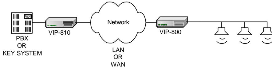
In this example, the VIP-810 was connected to the data network jack already installed and now the network connected telephone can reach into the existing Valcom Page Controller to access all call priority paging. This configuration could be used at a guard shack where network access is available, but not telephone.
