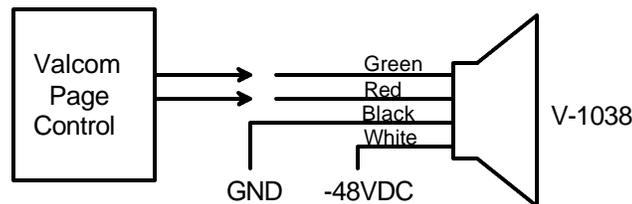
Used to expand loudspeaker paging capabilities
