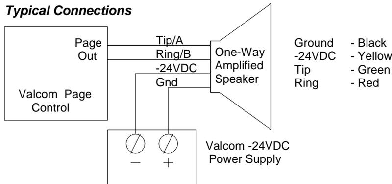
**NOTE:** Do not connect this speaker directly to 25/70/100V amplifier as damage to both the amplifier and speaker may occur. A V-1095 may be used to allow the use of Valcom self-amplified speakers on 70V speaker lines.
